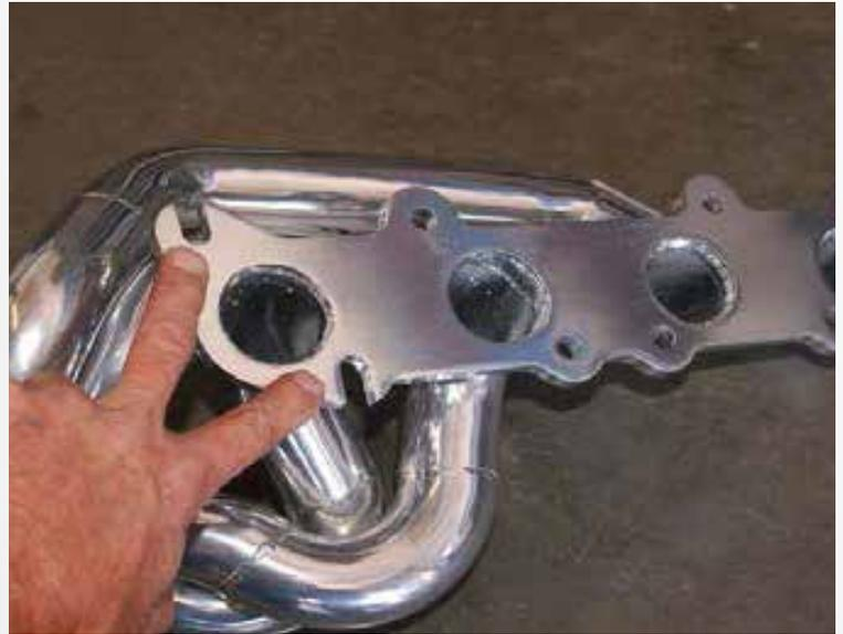
Looking at the BBK Header Flange, remove the studs that correspond with the notches in the flange. On the driver side it's the two most rear studs. Those will be replaced with supplied bolts.
