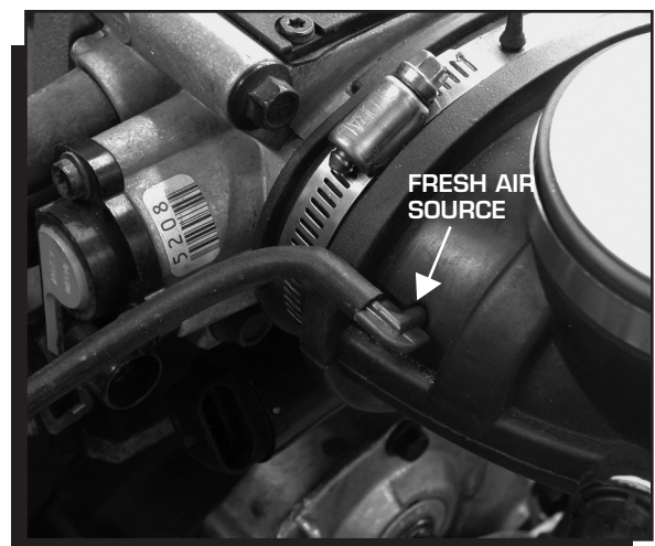
Figure 9 Installing the Fresh Air Line.
