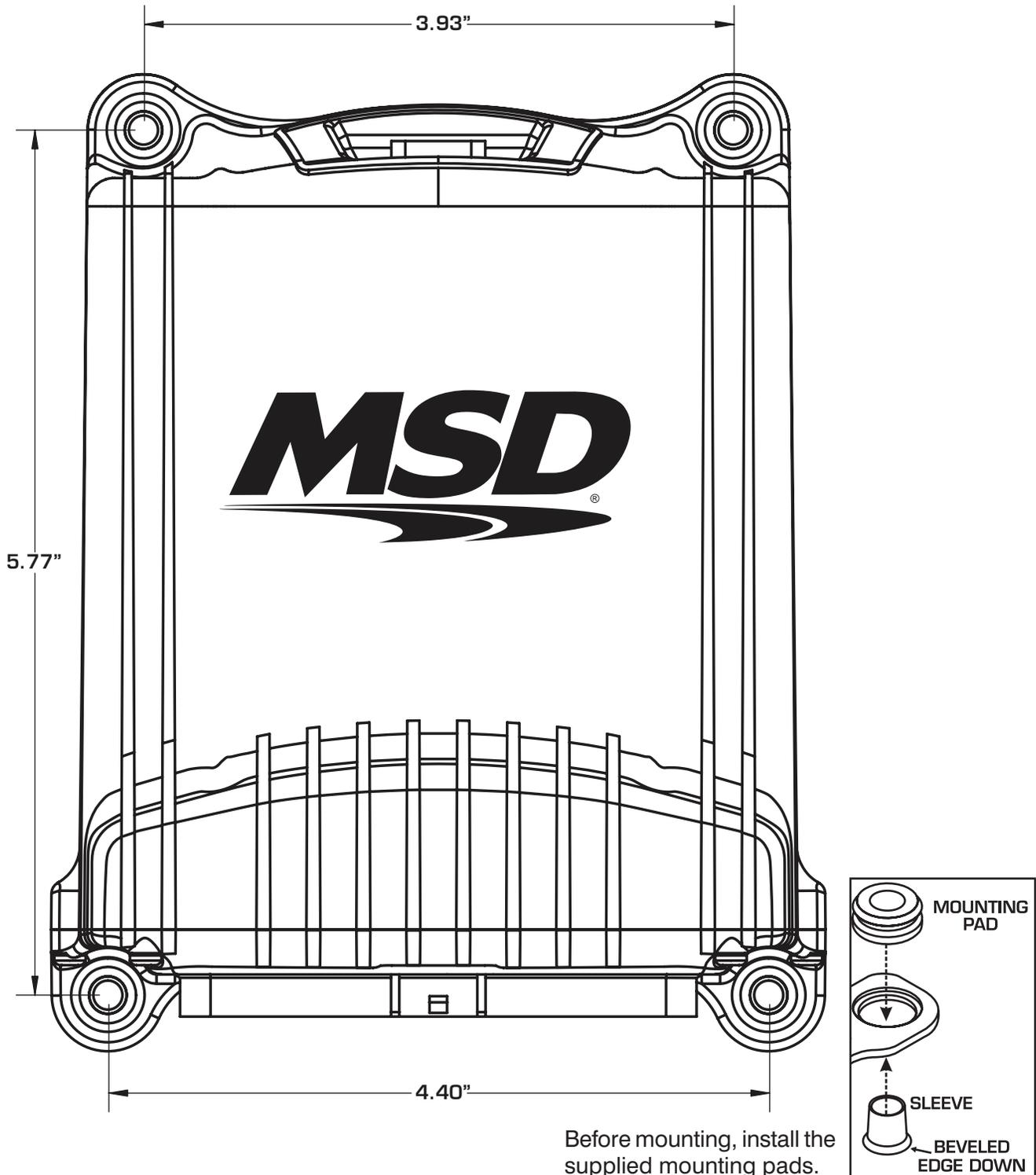
Before mounting, install the supplied mounting pads.
