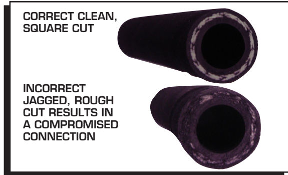
Figure 5 Severing the Hose Properly.
