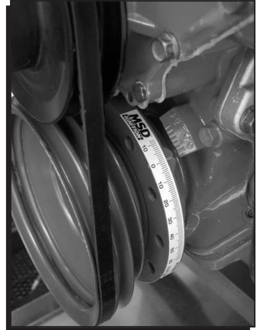
Figure 9 The Timing Tape Installed.
