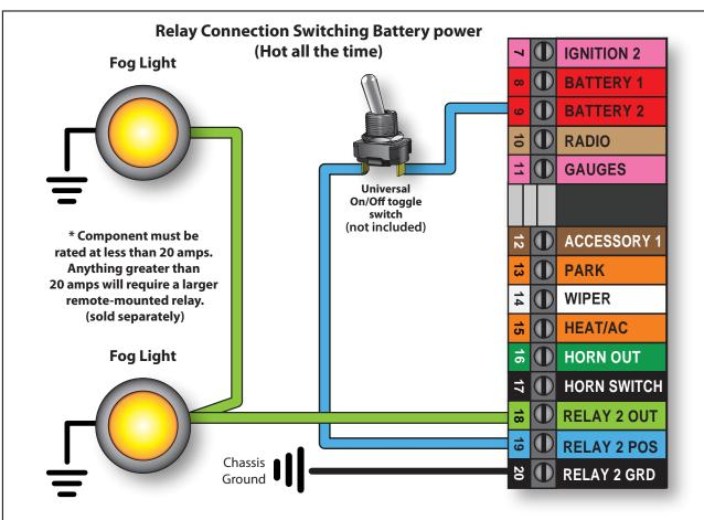
Fog lights are used for the example but any component rated under 20 amps will be acceptable.
