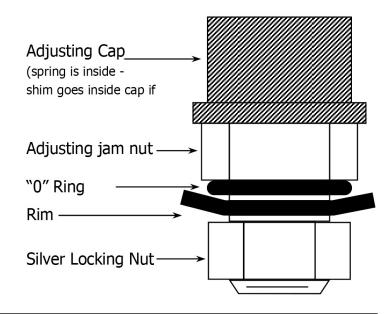
Use the low pressure springs to convert TIRELIEFS to 3 - 15 psi pressure range. Simply loosen the thin jam nut, unscrew the cap and replace the spring. Reassemble, and adjust.
