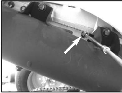
7. Remove the bolt that goes into the side of the air box (exhaust side).
