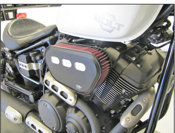
18. Install the front plate and filter assembly onto the back plate and secure to it to the back plate with the provided hardware. NOTE: Be sure the filter seats into the front and back plate correctly as the assembly is tightened.
