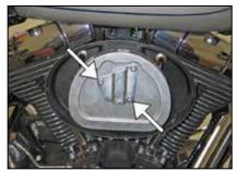
3. Remove the three bolts which secure the air filter to the filter base and then remove the air filter along with the crankcase breather tubes.
