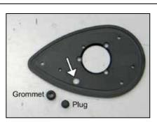
7. On vehicles equipped with a EVAP vent line, install the provided grommet into the hole shown. On vehicles not equipped with an EVAP vent line, install the provided plug into the hole shown from the back side of the base plate.
