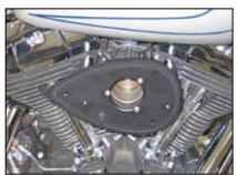
11. Install the three filter base plate mounting bolts into the base plate; install the remaining gasket and one drop of thread locker on each bolt. Secure the filter base plate to the Breather plate as shown. NOTE: On vehicles equipped with an EVAP vent line, connect the vent line to the base plate with the 90° hose mender and hose provided. Trimming of the hose will be necessary.
