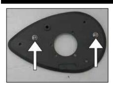
10. Apply one drop of thread locker to the two bolts provided and then secure the bolts and flat washers to the back side of the filter base plate as shown.
