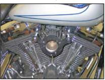
9. Install the crankcase breather plate along with the two remaining o-rings, mounting bolts (with one drop of thread locker) and throttle body gasket as shown.
