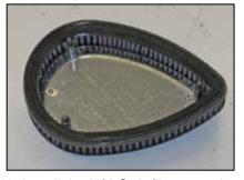
13. Install the K&N® air filter onto the top plate as shown.
