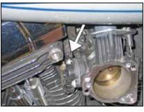
6. Using the provided tie wrap, secure the wiring pig tail to the throttle body wiring harness. **NOTE: On non-US models, a by-pass module**
