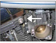
6. Using the provided tie wrap, secure the wiring pig tail to the throttle body wiring harness.
