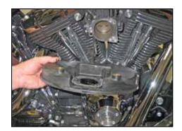
5. Remove the air filter base from the throttle body and unhook the wiring pig tail from the filter base. NOTE: K&N Engineering, Inc. recommends that customers do not discard the factory air intake components.
