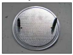
11. Apply thread locker to the two provided studs and then install the studs along with the lock washers onto the filter top plate as shown.
