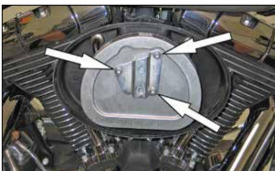
3. Remove the three bolts which secure the air filter to the filter base and then remove the air filter along with the crank case breather tubes.
