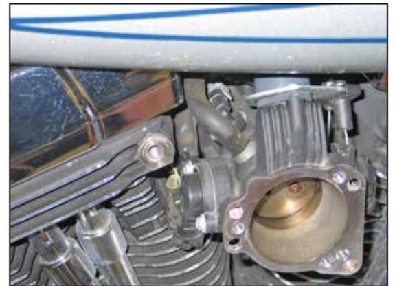
6. On Models equipped with the electrical pigtail, using the provided tie wrap, secure the wiring pig tail to the throttle body wiring harness.
