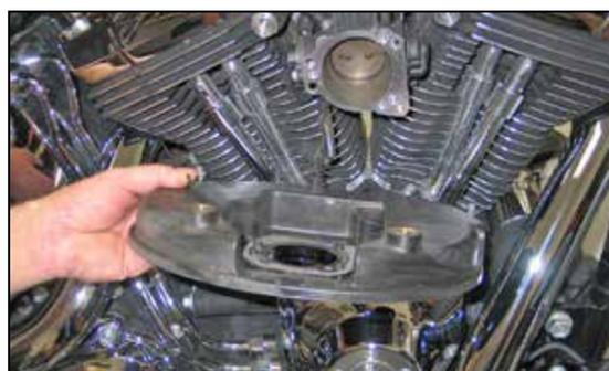
5. Remove the air filter base from the throttle body and unhook the wiring pig tail from the filter base.
