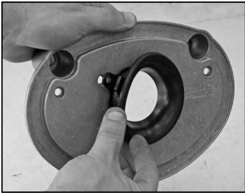
7. Install the velocity stack onto the supplied back plate.
