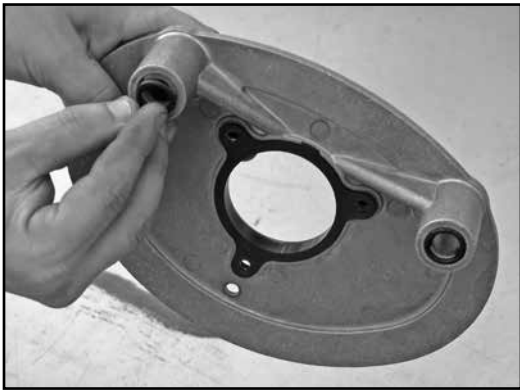
9. Install the two o-rings into the back plate standoffs.
