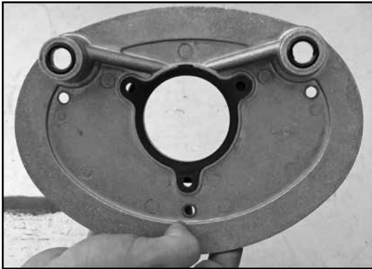
8. Align the holes on the velocity stack with the bolt holes in the back plate.
