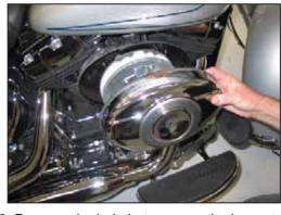
2. Remove the bolt that secures the bonnet to the filter assembly and then remove the bonnet from the vehicle.
