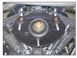
13. Install the base plate onto the throttle body and secure with the provided factory breather bolts and throttle body bolts.
