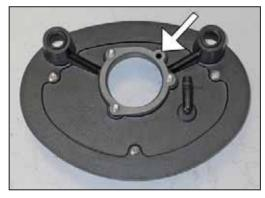
12. Install the provided gasket onto the base plate as shown.
