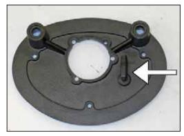
8. On models equipped with an EVAP vent line, drill a ½"ID hole in the base plate at the location marked in step #7. Then install the provided grommet and 90° hose mender as shown.
