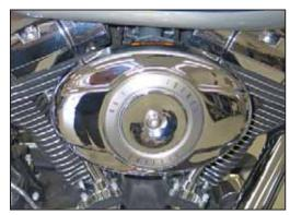
15. Install the filter bonnet onto the air filter and secure with the factory bolt.
