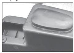
16. Install the small plug into the air cleaner housing.
