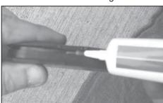
15. Apply sealing grease into the groove of the small plug.
