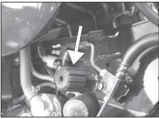
5. Lift the fuel tank off of the tank cushions. NOTE: The fuel tank does not need to be completely removed, only tilt up for air cleaner housing removal.
