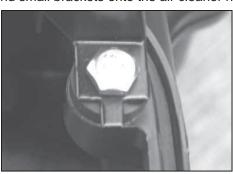
21. Make sure that a flat side of the Hex bolt is even with the tab on the bracket.
