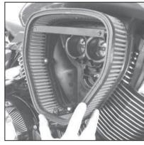
26. Install the K&N® air filter onto the air cleaner housing.
