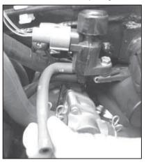
11. Remove the diaphragm hose from the valve assembly.
