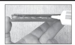
17. Apply sealing grease into the groove of the large plug.
