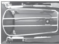
2. On models with optional solo rider rear carriers, remove the screws that hold the carrier to the rear fender.
