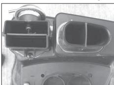
14. Remove the duct screw. Gently pry the ducts off of the air cleaner housing.
