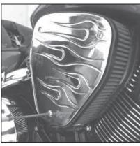
27. Install the front plate on the K&N® air filter NOTE: Make sure the front plate is completely seated onto the K&N® air filter.
