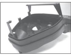
20. Using the supplied Hex bolts, install the large and small brackets onto the air cleaner housing.
