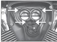
8. Remove the four air funnel screws and remove the air funnel.
