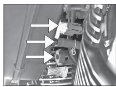
9. Gently pry the air cleaner housing from the mounting grommet. Disconnect the sensor and all of the breather tubes from the back of the air cleaner housing.
