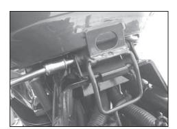
4. Remove the fuel tank hinge bolt.
