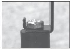
22. Bend the tab on the bracket up. This will keep the Hex bolt from backing out.
