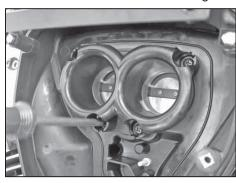
24. Reinstall the air funnel and tighten the screws.
