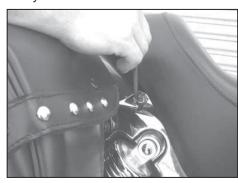
1. Remove the seat bolts (one on each side)
