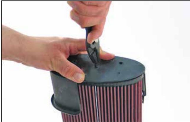
4. Install the top plate from the OE filter onto the K&N® filter. Using a pair of pliers, pull the rubber tip from the K&N® filter through the hole on the filter top plate.
