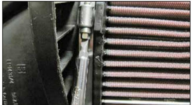
9. Re-position clamp to ensure correct placement onto flange of K&N® filter and tighten.
