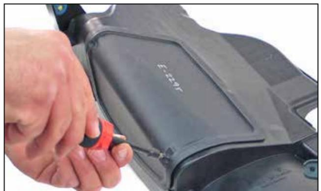
11. Install air filter cover and fasten screws.
