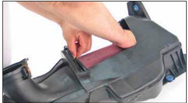
8. Slide filter onto flange portion of OE air box. You may be required to place one hand on the top of the filter and push. Use pull tabs built into filter base to assist pulling filter flange onto air box flange until filter is seated.
