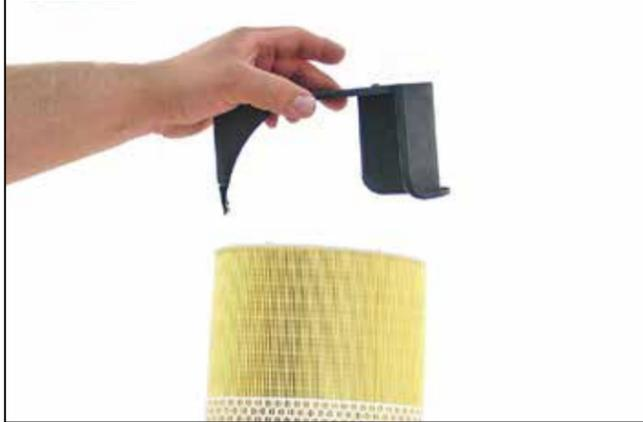
3. Remove the dirty air filter and remove the screw (which will not be re-used) that fastens the top plate to the filter and depress the four tabs to release the top plate from the filter.
