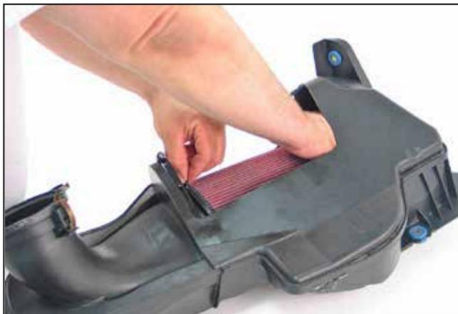
6. Place K&N® filter top side first into air box. **NOTE: make sure that the filter lid is orientated correctly so that the screw hole is reused on step 9.** Position filter so that it can be pulled toward air box flange.
