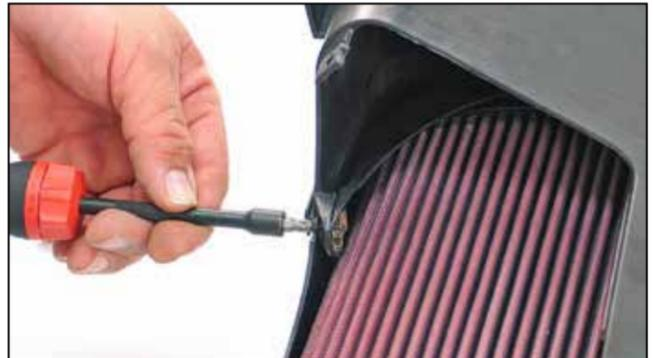
10. Once K&N® filter is seated onto air box flange and clamp is tight, install screw that retains filter in place.
