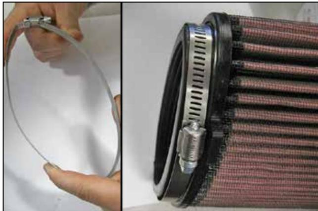
5. Squeeze the clamp supplied with the K&N® filter as shown to conform to the filter base flange and install hose clamp onto air filter
