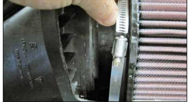
7. With filter resting in air box, loosen clamp completely from the air filter. Filter cannot be installed with the clamp tightened onto air filter flange.
