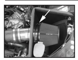
Step 20 Install the filter and fully tighten the clamp.
