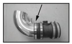
Step 14 Install the large intake tube with the MAFS pointing towards the intake tube.
