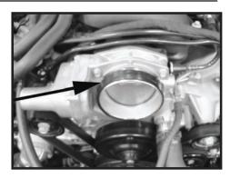
Step 16 Place the thin spacer on the throttle body.
