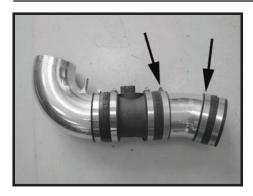
Step 15 Install the small intake tube with the longer end closer to the MAFS. Take note of the orientation of the tube, this may be rotated slightly once the assembly is installed in the vehicle.
