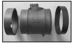
Step 12 Install the thick rubber spacer on end of the MAFS that the arrow is pointing too. Install the thin rubber spacer on the opposite end of the MAFS.
