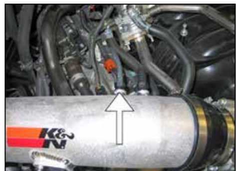
28. Reconnect the fuel pressure regulator vent line to the NPT fitting as shown.
