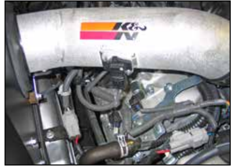
30. Reconnect the mass air sensor electrical connection.
