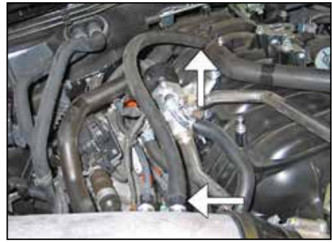
29. Connect the provided crankcase vent line to the NPT fitting and then to the factory TEE fitting on the intake plenum as shown.
