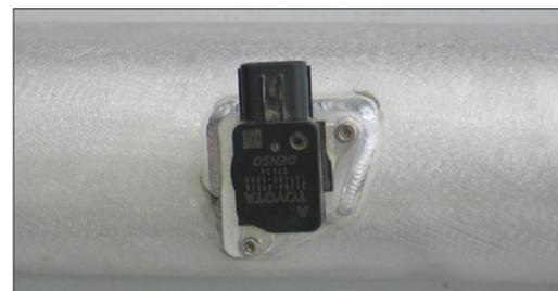
23. Install the mass air sensor into the K&N® intake tube and secure with the provided hardware.
