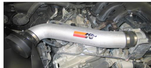
26. Install the K&N® intake tube into hump hose at the filter adapter and then into the silicone hose at the throttle body, align the tube for proper fit and then tighten the hose clamps.
