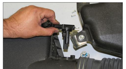
22. Remove the screws which secure the mass air sensor to the factory air box and then remove the mass air sensor from the air box.
