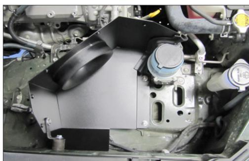
19. Set the heat shield onto the rubber mounted studs and secure with the provided hardware.
