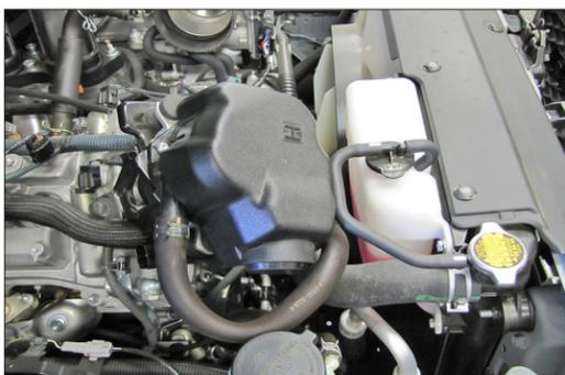
11a. Lift up the air injection pump, disconnect the electrical connection and then set the air injection pump over to side.
