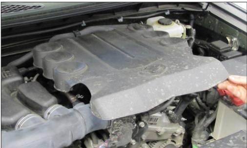
2. Lift up the engine cover to dislodge it from the mounting grommets and then remove the cover from the vehicle.
