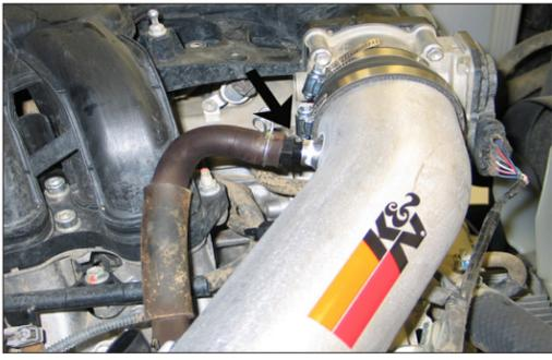
27. Connect the crank case vent line to the 5/8 vent fitting and secure with the factory spring clamp.
