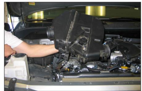
8. Lift up the air box assembly and disconnect the fuel pressure vent line and then remove the complete air box assembly.
