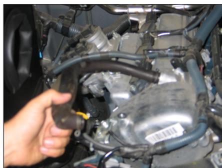
19. Reverse the crank case vent hose and reinstall it back onto the valve cover.
