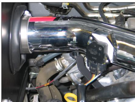
32. Reconnect the Mass air sensor electrical connection.
