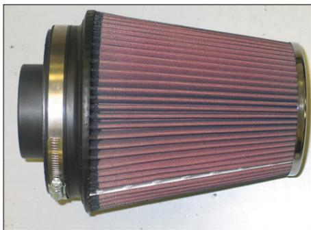
28. Install the filter adapter into the K&N® air filter and secure with the provided hose clamp.
