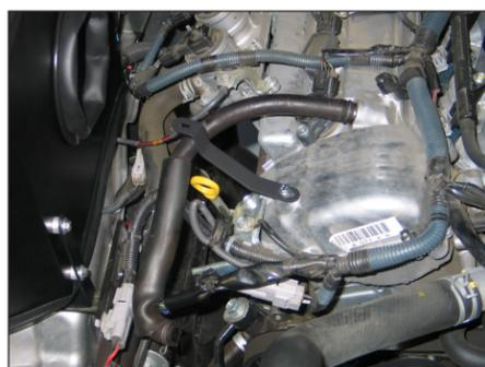
20. Install the tube mounting bracket (070088) onto the valve cover using the provided hardware as shown.
