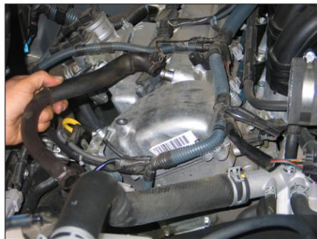
18. Remove the crank case vent hose from the valve cover.
