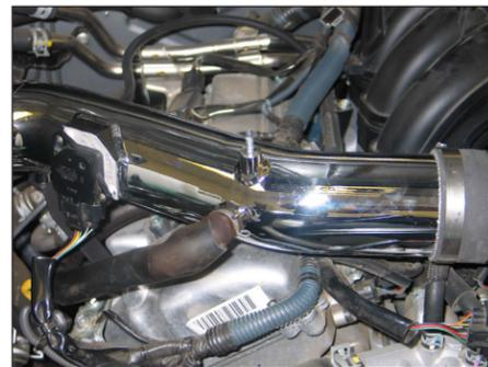
27. Install the engine cover mounting stud into the K&N® intake tube as shown.
