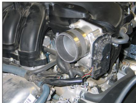
21. Install the provided silicone hose (08711) onto the throttle body and secure with the provided hardware.
