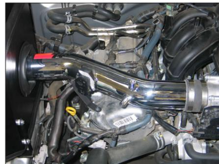
25. Install the K&N® intake tube assembly into the silicone hose at the throttle body and align with the tube mounting bracket, then secure with the provided hose clamp and hardware.
