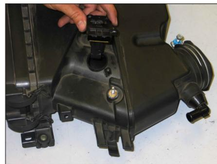
22. Remove the mass air sensor from the stock air box as shown.
