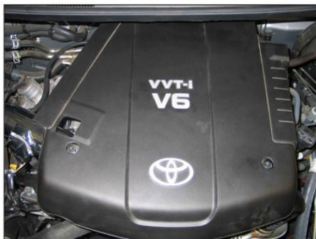
33. Reinstall the engine cover and secure with the factory mounting nuts.
