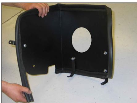
13. Install the provided edge trim around the heat shield as shown.
