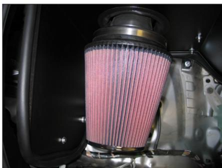
30. Install the filter assembly onto the K&N® intake tube and secure with the provided hose clamp.
