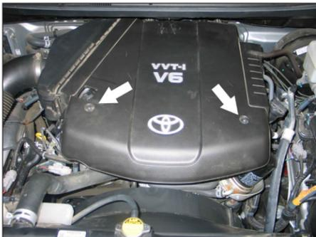
2. Remove the two nuts shown that secure the engine cover and then remove the engine cover.
