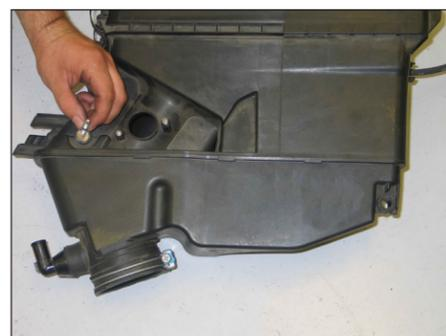
24. Remove the engine cover mounting stud from the factory air box.
