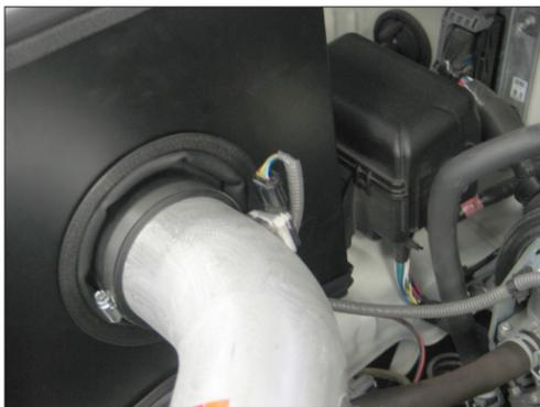
28. Reconnect the mass air sensor electrical connection as shown.
