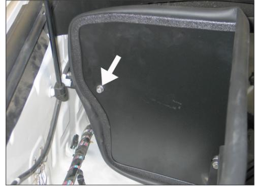
19. Secure the rear of the heat shield to the bracket installed in step #11.
