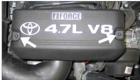
3. Remove the two nuts that retain the engine cover. Remove the engine cover from the engine.
