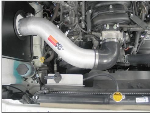
24. Install the K&N® intake tube into the silicone hose at the throttle body and align with the mounting bracket installed during step #10. Secure the intake tube with the hose clamp and hardware provided.
