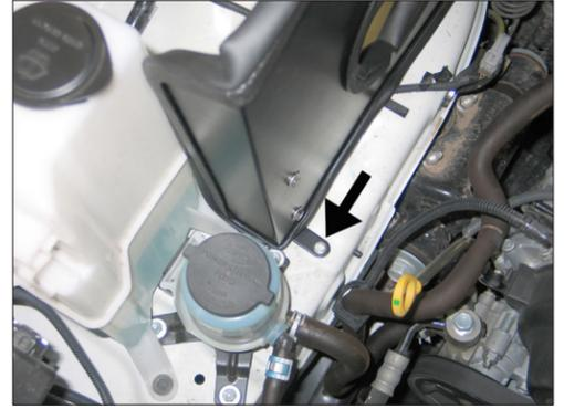
18. Secure the front heat shield bracket to the front air box mounting location with the provided hardware.
