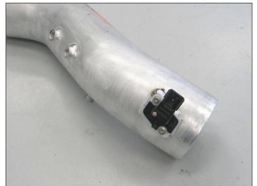
22. Install the mass air sensor into the K&N® intake tube and secure with the provided hardware.
