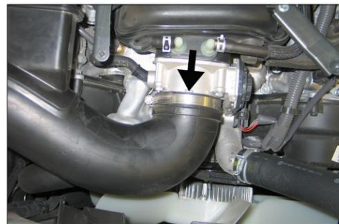
4. Loosen the hose clamp that secures the stock intake tube to the throttle body.
