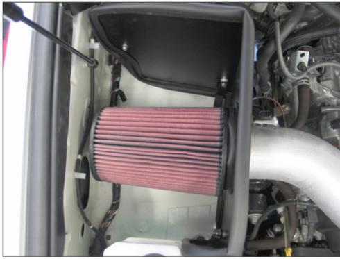
27. Install the K&N® air filter onto the K&N® intake tube and secure with the provided hose clamp.
