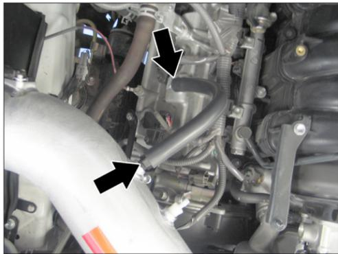
25. Install the provided crank case vent hose onto the valve cover fitting, and then connect the open end to the NPT fitting installed into the K&N® intake tube as shown.
