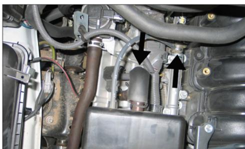
5. Disconnect the fuel pressure regulator hose from the fuel pressure regulator. Disconnect the crank case vent hose from the valve cover.
