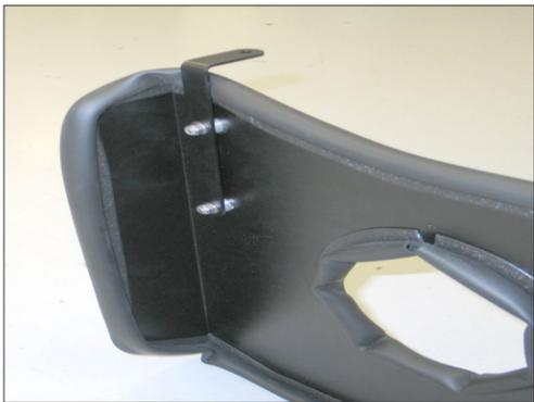
12. Install the long "L" bracket (#070902) onto the heat shield with the provided hardware as shown.
