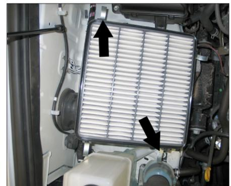
7. Remove the two factory bolts that secure the lower air box to the inner fender.
