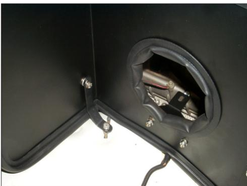
17. Set the heat shield into position on the inner fender. Secure the "C" bracket to the ground strap location.
