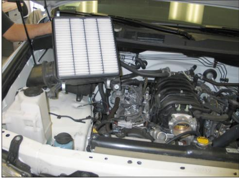
8. Lift the lower air box up, releasing it from the inner fender mounting grommet and fresh air duct. Remove the lower air box from the vehicle.
