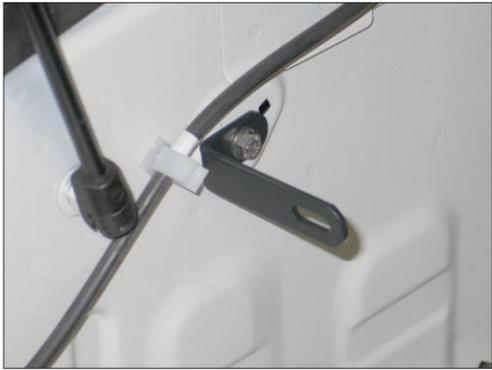
9. Install the small "L" bracket (#070742) onto the inner fender, behind the hood support. Secure with the provided hardware as shown.
