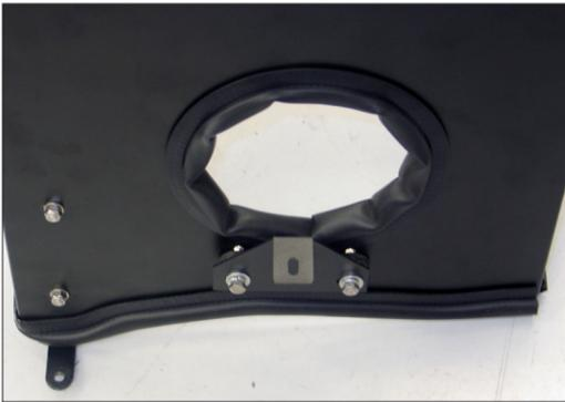
15. Install the tube mounting bracket assembly onto the heat shield as shown using the provided hardware.
