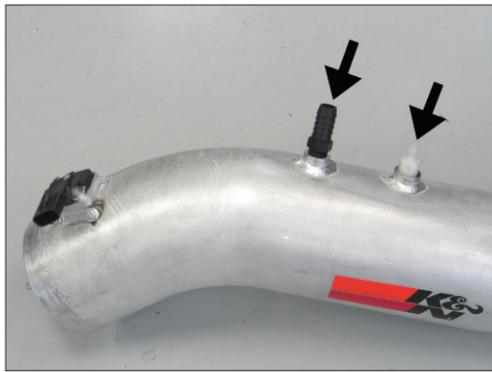
23. Install the provided 1/4" npt fittings into the K&N® intake tube as shown.
