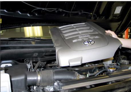
2. Lift up the front of the engine cover and then unhook it from the rear and remove it from the vehicle.
