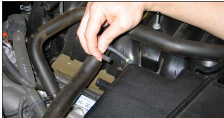
5. Disconnect the fuel pressure regulator vent hose from the stock intake tube as shown.
