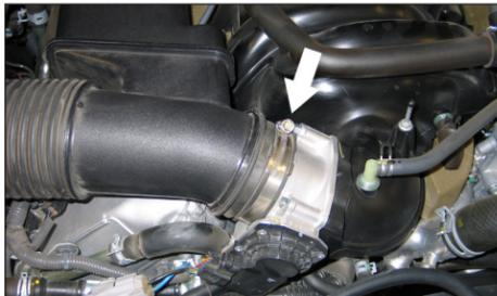
6. Loosen the hose clamp which secures the stock intake tube to the throttle body.
