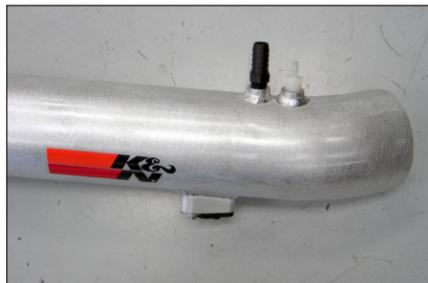
20a. Install the two provided 1/4" npt fittings into the K&N intake tube as shown. **NOTE: Plastic NPT fittings are easy to cross thread. Install the vent fitting "hand" tight, then turn it two complete turns with a wrench.**
