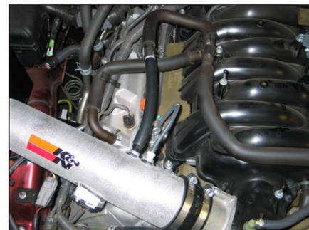
25. Connect the hose mender from the crank case vent hose assembly into the factory crank case vent hose and secure with the factory spring clamp. Then connect the open end to the K&N intake tube as shown.
