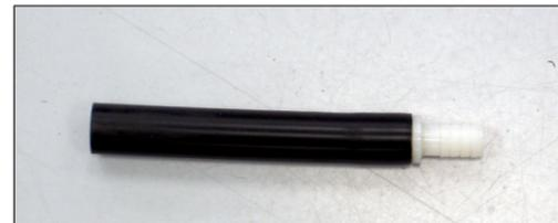
24. Install the provided hose mender into the provided crank case vent hose.
