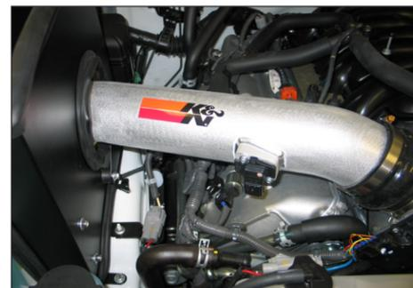
22. Install the K&N intake tube into the silicone hose at the throttle body and align with bracket installed on the heat shield. Align tube and heat shield then tighten the heat shield and secure the intake tube with the provided hardware.
