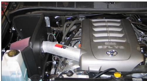
31. Reconnect the vehicle's negative battery cable. Double check to make sure everything is tight and properly positioned before starting the vehicle.
