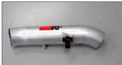
20. Install the mass air sensor into the K&N intake tube using the hardware provided.
