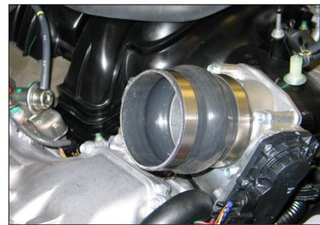
21. Install the silicone hose (084057) onto the throttle body as shown and secure with the provided hose clamp.
