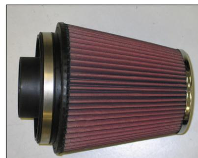
26. Install the filter adapter into the K&N air filter as shown and secure with the provided hose clamp. **NOTE: Drycharger air filter wrap; part # RF-1042DK is available to purchase separately. To learn more about Drycharger filter wraps or look up color availability please visit <http://www.knfilters.com>.**
