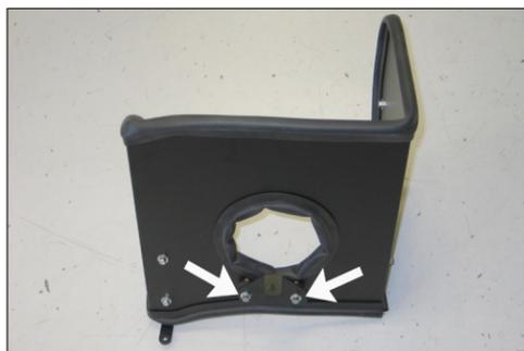
14a. Install the tube mounting bracket on the heat shield as shown using the provided hardware. **NOTE: Be sure to place the provided rubber mounted studs between the heat shield and bracket. Do not completely tighten at this time.**
