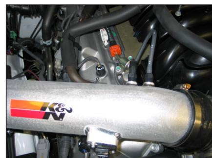
23. Connect the factory fuel pressure vent hose to the K&N intake tube as shown.
