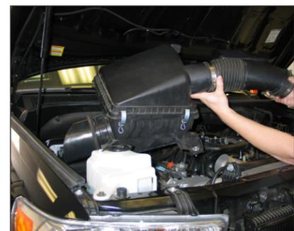
8. Remove the complete stock intake assembly from the vehicle as shown.
