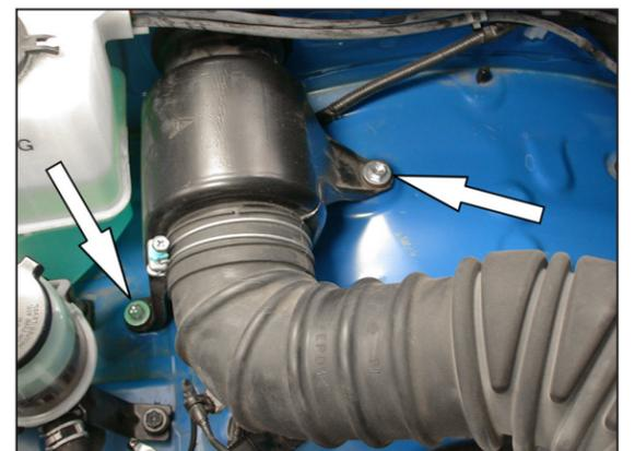
6. Remove the two intake resonator mounting bolts shown.
