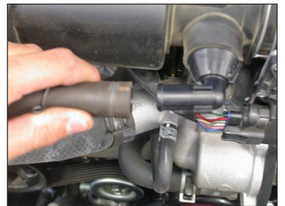
5. Slide the spring clamp back and then disconnect the crank case ventilation hose from the fitting on the factory air box.
