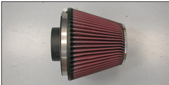
24. Install the provided filter adapter into the K&N® filter as shown and secure with the provided hose clamp.
