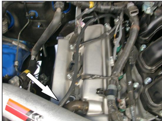
28. Install the provided vent hose onto the fuel pressure regulator and then onto the K&N® intake tube as shown.
