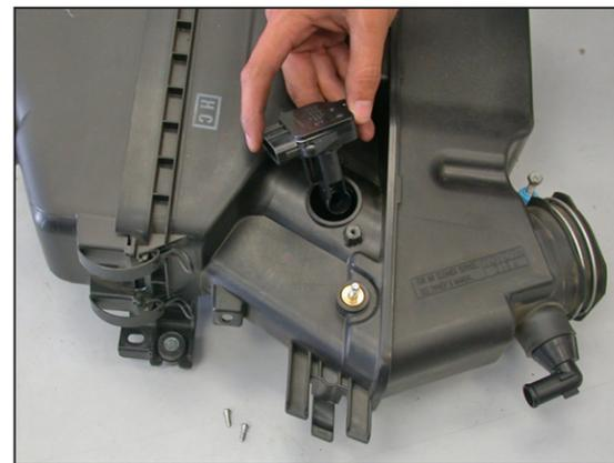
17. Remove the two screws that secure the mass air sensor to the air box and then remove the mass air sensor from the air box.
