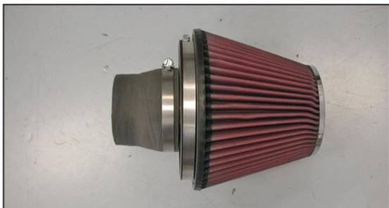
25. Install the provided silicone hose (08724) onto the K&N® filter assembly and secure with the provided hose clamp.
