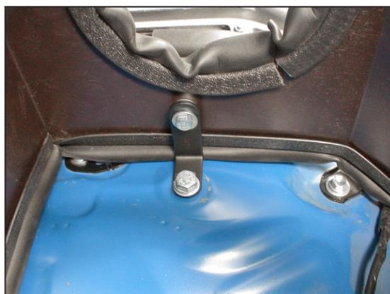
16. Secure the bottom of the heat shield to the inner fender with the small "L" bracket.
