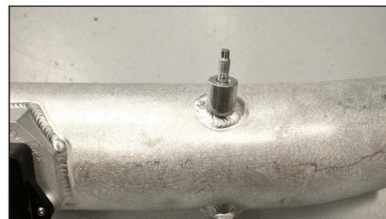
20. Install the engine cover mounting stud into the K&N® intake tube as shown.
