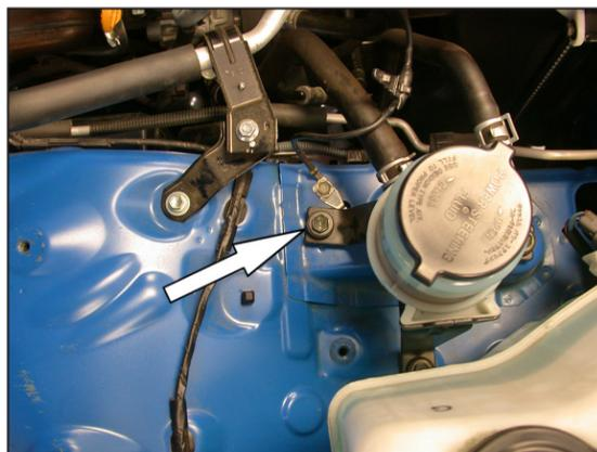
13. Remove the power steering reservoir mounting bolt shown.
