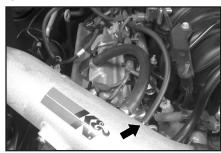
18. Connect the supplied fuel pressure regulator vent hose to the fuel pressure regulator and then onto the K&N<sup>®</sup> intake tube as shown.
