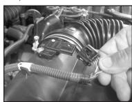
3. Disconnect the mass air sensor electrical connection, then release wire loom from air box.
