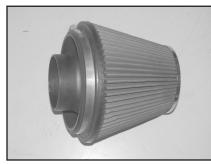
20. Install the filter adapter into the K&N<sup>®</sup> air filter as shown and secure with the provided hose clamp.
