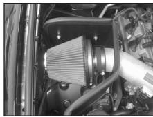
22. Install the air filter assembly onto the KN<sup>®</sup> intake tube as shown and secure with the provided hose clamp.
