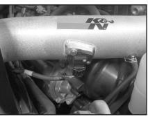
26. Reinstall the throttle body cover as shown.
