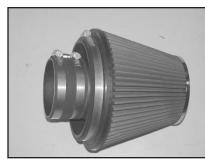
21. Install the silicone hose (08698) onto the K&N<sup>®</sup> air filter assembly and secure with the provided
