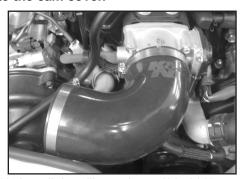
13. Install the silicone hose (084089) onto the throttle body and secure with the provided hose clamp.
