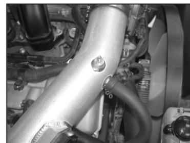
25. Install the original crank case vent hose onto the valve cover, then connect the crank case vent hose onto the K&N® intake tube.
