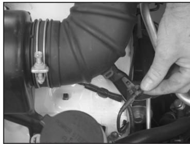
4. Pull the wire harness clip up to release it from the intake tube.
