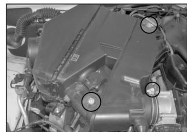
10. Loosen the hose clamp at the throttle body, then remove the two bolts that secure the air box to the engine.
