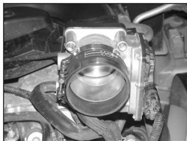
17. Install the silicone hose (08434) onto the throttle body with the provided hose clamps as shown.
