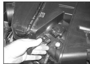
7. Disconnect the two mass air wire harness retaining clips from the air box, then disconnect the mass air sensor electrical connection.
