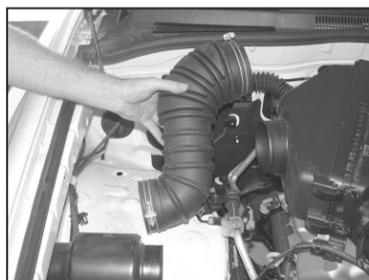
5. Remove the intake tube from the vehicle as shown.
