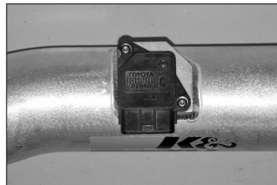
22. Secure the mass air sensor to the K&N® intake tube using the provided bolts as shown.
