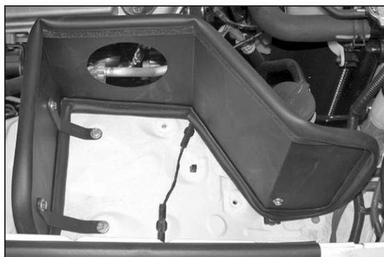
17. Install the heat shield onto the vehicle, then secure the brackets with the provided hardware.
