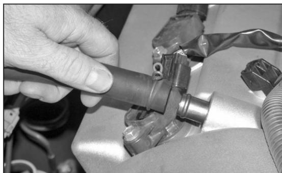
19. Flip the crankcase vent hose around and reconnect the opposite end of the hose to the valve cover.
