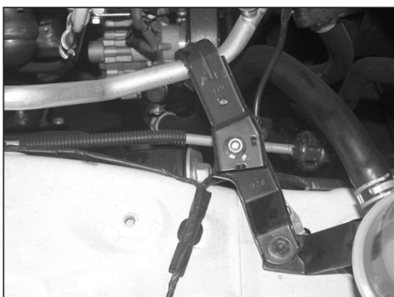
13. Rotate the A/C mounting bracket onto the power steering reservoir, then secure it using the bolt from the previous step. Tighten the A/C mounting nut.
