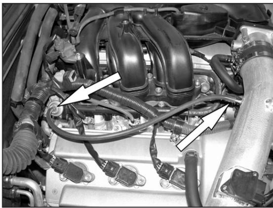
27. Remove the stock vacuum hose from fuel pressure regulator. Install the provided silicone hose, attaching the hose to the fuel pressure regulator and the K&N® intake tube nipple.
