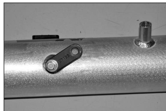
25. Install the tube mounting bracket (07133) onto the K&N® intake tube as shown.
