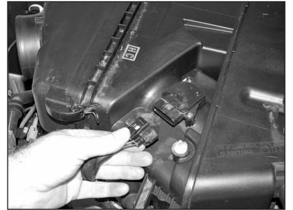
7. Disconnect the two mass air wire harnesses retaining clips from the airbox, then disconnect the mass air sensor electrical connection.
