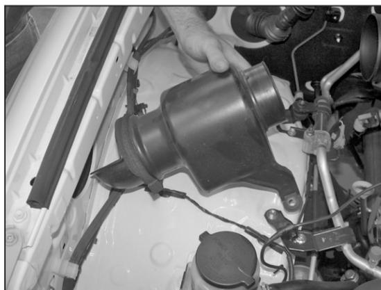
6. Remove the two bolts that secure the resonator to the inner fender, then remove resonator from vehicle as shown.
