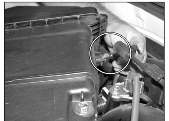
9. Remove the fuel pressure regulator hose from the back side of airbox.
