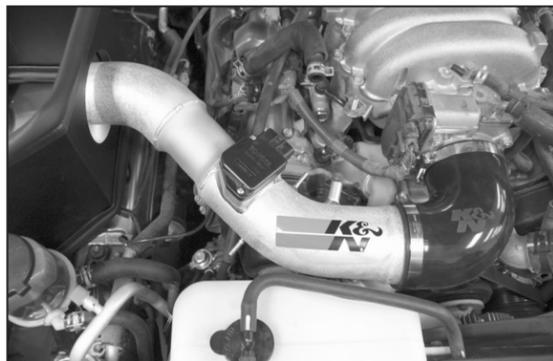
16. Install the K&N® intake tube into the silicone hose at the throttle body and align the mounting boss with the mounting bracket installed in step #12. Secure with the provided hardware.
