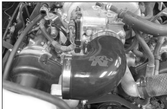
13. Install the provided silicone hose (084095) onto the throttle body with the provided hose clamp.
