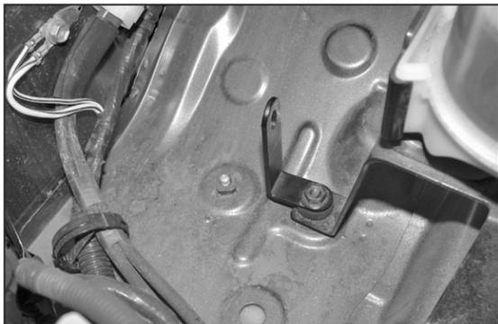
8. Remove the 12mm bolt that retains the power steering reserve to vehicle then mount the provided bracket (07158) onto the vehicle with the bolt that was removed.
