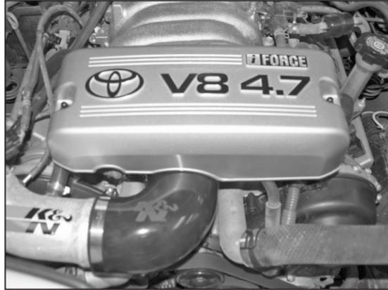
26. Reinstall the throttle body cover as shown.
