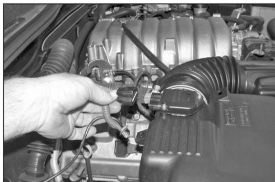
3. Disconnect the mass air sensor electrical connection, then release wire loom from air box.
