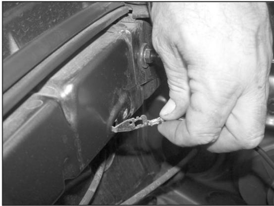
23. Disconnect the ground strap that's attached to the mass air sensor wiring harness at the inner fender as shown.
