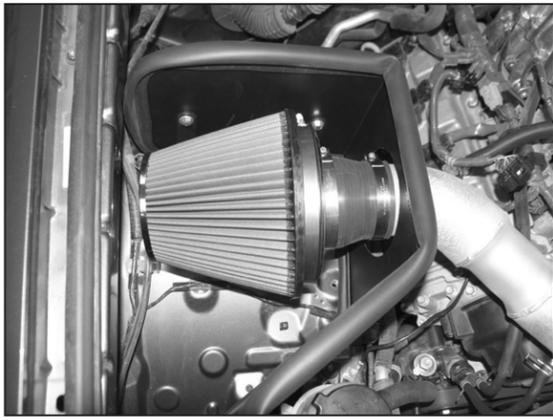
22. Install the air filter assembly onto the K&N® intake as shown and secure with the provided hose clamp.
