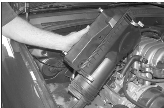
7. Remove the three bolts that retain the air box to vehicle, then remove the air box.
