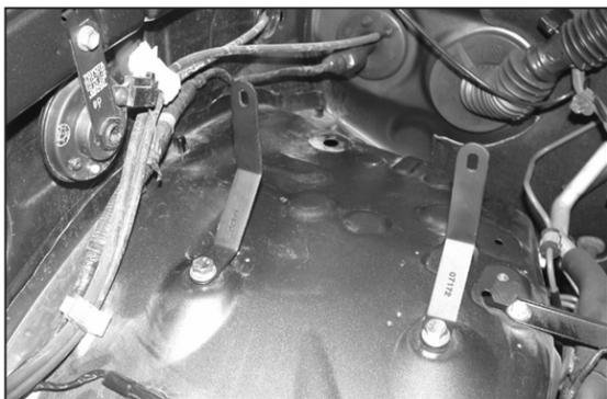
9. Mount the two provided brackets onto the vehicle with the provided hardware.
