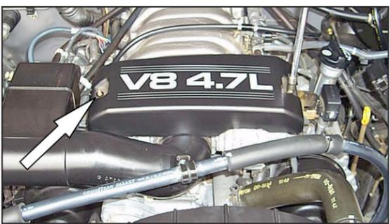
3. Loosen and remove the acorn nuts that secure the throttle body cover, then remove the cover.
