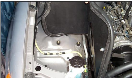
15. Install the heat shield onto the rubber mounted studs as shown above.
