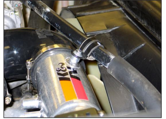
21. Reconnect the A/C line to the K&N® intake tube using the original bolt removed in step #4.
