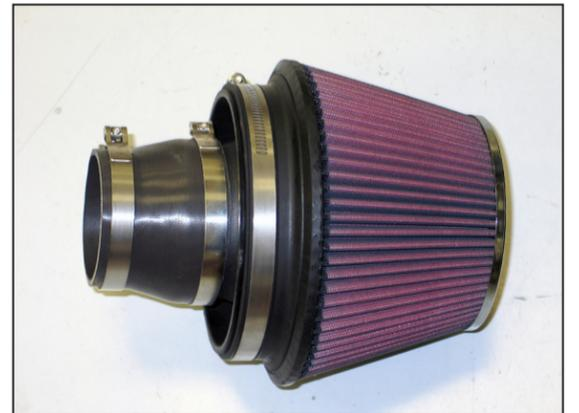
25. Install the silicone hose (084091) onto the filter adapter and secure with the provided hose clamp as shown.
