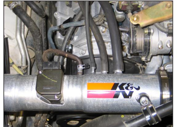
23. Install the one factory P/S vent line, crank case vent line, EVAP vent line, and fuel pressure vent line onto the K&N® intake as shown.
