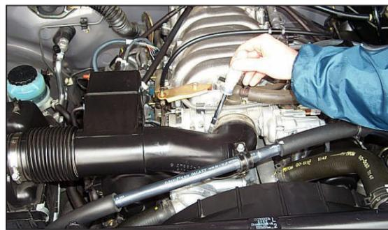
5. Loosen the hose clamp at the throttle body.
