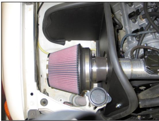
26. Install the air filter assembly onto the K&N® intake tube as shown.
