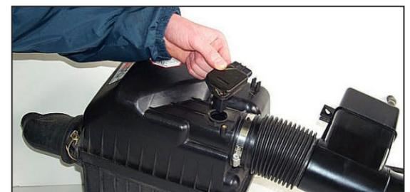
9. Loosen and remove the two screws that secure the mass-air sensor, then remove the mass-air sensor.
