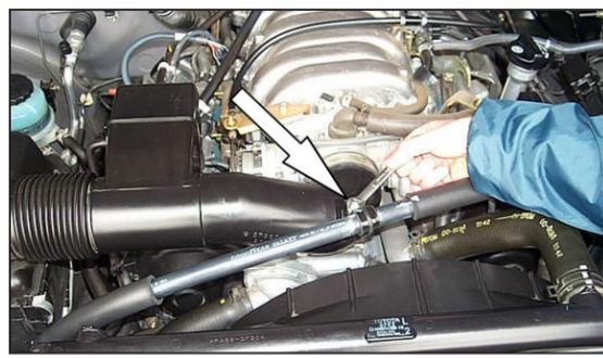
4. Loosen and remove the bolt that secures the AC line to the stock intake tube.
