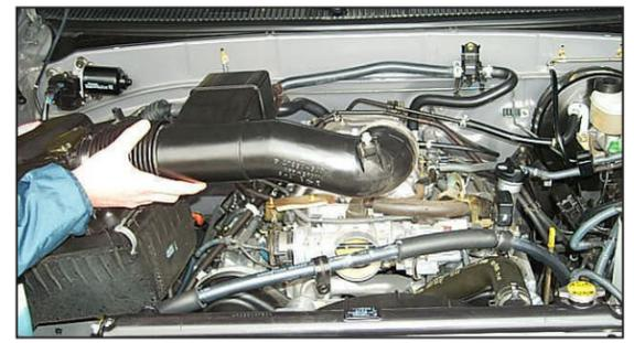
8. Remove the complete air induction system.
