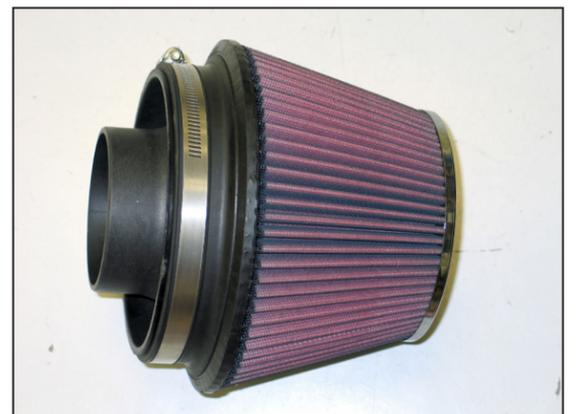
24. Install the filter adapter into the air filter as shown and secure with the provided hose clamp.
