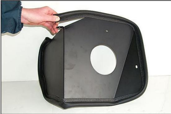
11. Apply the edge trim to the K&N® heat shield as shown above, trim if needed.
