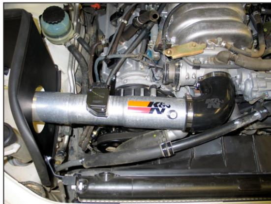
20. Install the K&N® intake tube into the silicone hose at the throttle body and then align the tube mounting bracket with the threaded boss on the engine valve cover. Secure the tube with the provided hardware and tighten the hose clamp.
