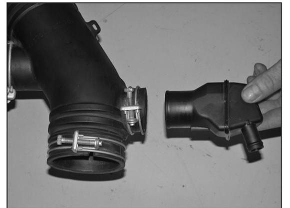
7. On vehicles equipped with the crank case vent resonator chamber, loosen the hose clamp which secures the chamber to the intake tube and remove the chamber from the tube as shown.
