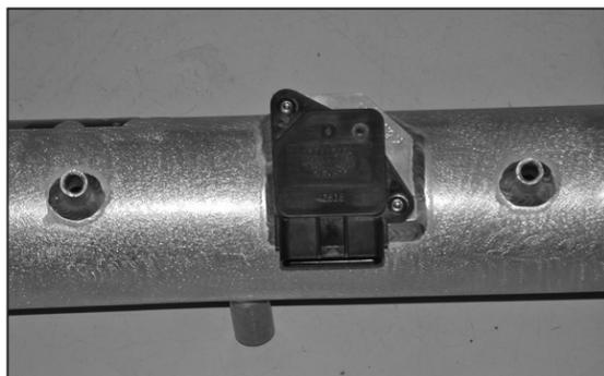
12. Install the mass air sensor into the K&N® intake tube and secure with the provided hardware.
