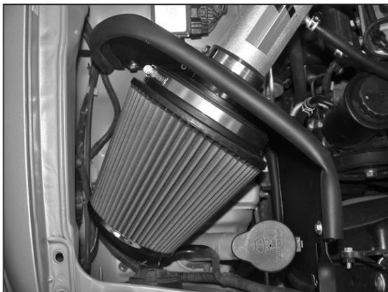
26. Install the air filter assembly onto the K&N® intake tube and secure with the provided hose clamp.
