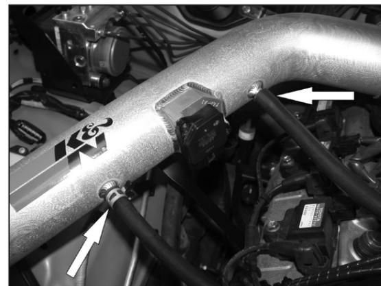
20. Install the provided silicone hose onto the engine and connect it to the K&N® intake tube as shown. Then attach the vent line from EVAP canister to the K&N® intake tube as shown.
