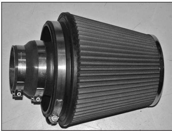
25. Install the silicone hose (084093) onto the air filter assembly as shown and secure with the provided hose clamps.
