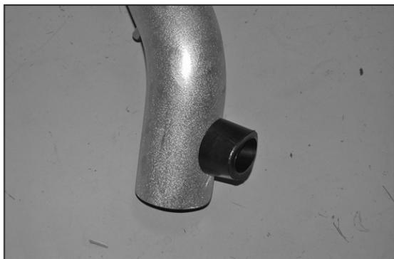
9. Install the resonator grommet provided into the 1-3/8" hole drilled in step #8 as shown.
