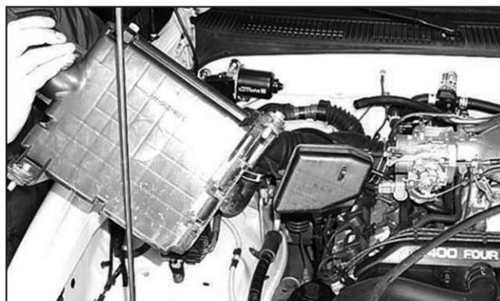
6. Remove the complete air intake system.
