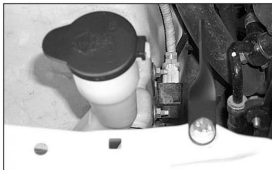
15. Install the twist bracket onto the existing air box-mounting hole with the provided hardware as shown. Do not tighten completely.
