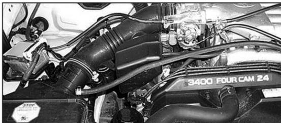
3. Disconnect the three hoses from the air box resonator and intake hose.
