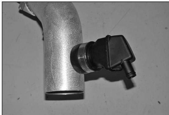
10. Install the crank case vent resonator into the grommet install in step #9 and secure with the provided hose clamp.
