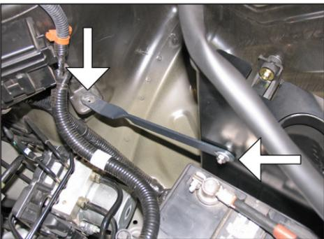
16. Install the heat shield mounting bracket #070840 onto the heat shield so that the other end of the bracket rests on the mounting tab on the strut tower as shown.
