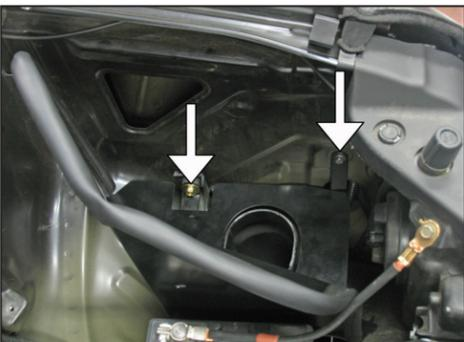
15. Install the heat shield assembly into the vehicle as shown. Secure the rear heat shield mounting bracket to the fresh air duct with the bolt removed in step #11. Secure the forward heat shield mounting bracket to the inner fender with the provided hardware as shown.
