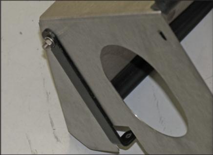
13. Install the provided "L" bracket #070026 onto the heat shield with the provided hardware as shown.
