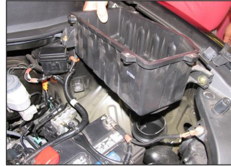
10. Remove the lower airbox housing as shown. **NOTE: K&N Engineering, Inc., recommends that customers do not discard factory air intake.**
