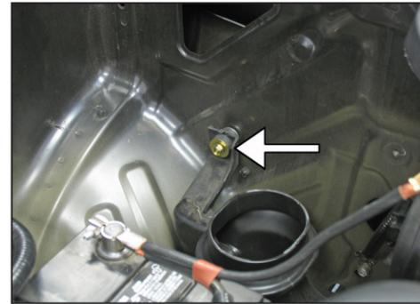
11. Remove the fresh air duct retaining bolt shown. **NOTE: This bolt will be reused.**
