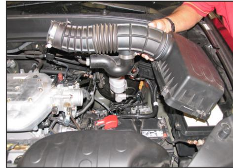
8. Remove the airbox lid and intake tube as shown.
