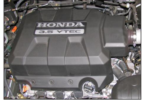
23. Reinstall the engine cover and secure in place with the three 1/4 turn fasteners.
