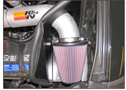
22. Install the K&N® air filter onto the intake tube as shown, and secure with the provided hose clamp.
