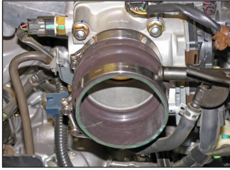
17. Install the silicone hose #08421 onto the throttle body with the provided hardware as shown.
