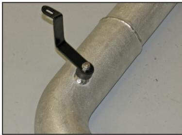
19. Install the tube mount bracket #010107 onto the K&N® intake tube as shown.
