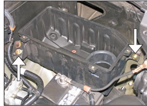
9. Remove the two lower airbox retaining bolts shown.
