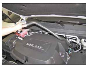
3. Disconnect the crank case vent hose from the intake plenum and then disconnect it from fitting on the valve cover and then remove it from the vehicle.
