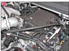
23. Install the crank case vent hose onto the fitting installed into the K&N® intake tube and then connect the hose mender into the fitting on the valve cover.
