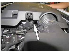
7. Loosen the hose clamp securing the intake plenum to the throttle body.
