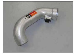
19. Install the mass air sensor into the  $K\&N^{\otimes}$  intake tube and secure with the provided hardware.
