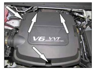
6. Loosen the two bolts that secure the rear off the intake plenum and remove the two forward bolts that secure the plenum.
