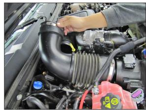
6. Remove the factory intake tube from the vehicle.
