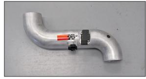
18. Install the MAF sensors into the K&N® intake tube and secure with the provided hardware. NOTE: On 2012 and earlier model year vehicles, it will be necessary to use the block off plate and gasket in place of mass air sensor.
