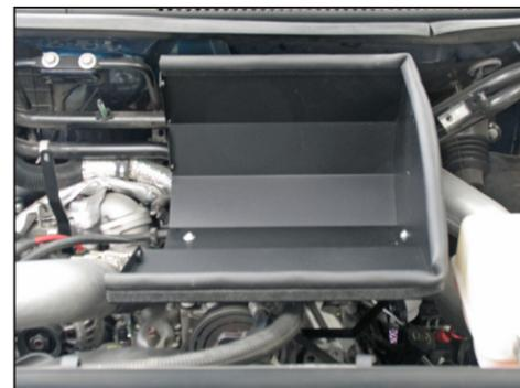
22. Install the heat shield onto the mounting bracket on the A/C compressor and secure with the provided hardware.
