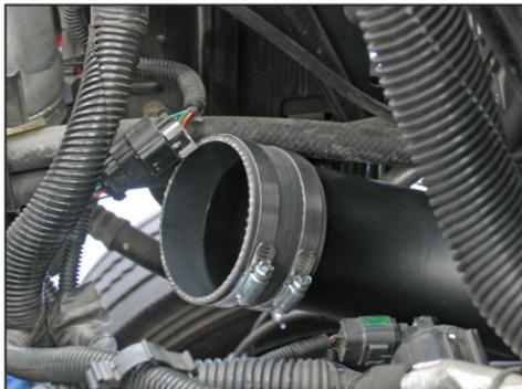
14. Install the silicone hose (08698) onto the primary intake tube and secure with the provided hose clamp.
