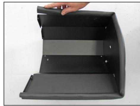
20. Install the long edge trim onto the heat shield as shown.
