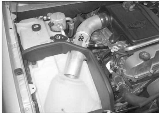
15. Install the K&N® intake tube assembly into the silicone hose at the throttle body and align it with the mounting bracket installed in step #12. Then secure the tube with the provided hose clamp and hardware.
