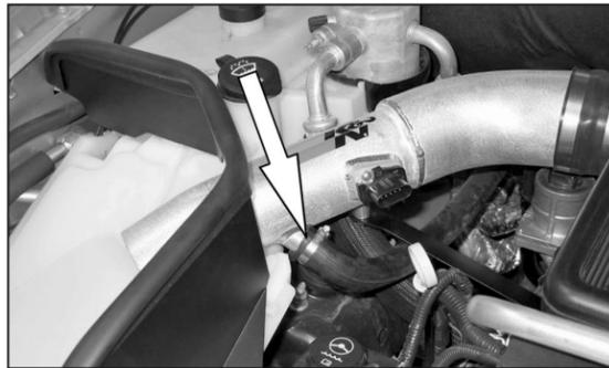
17. Cut the air injection hose at the location marked in step #16. Then install the hose onto the K&N® intake tube and secure with the provided hose clamp.
