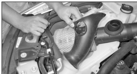
6. Remove the fresh air supply duct from the lower air box housing as shown.
