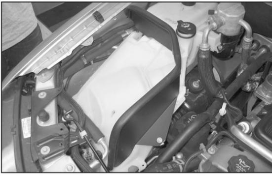
10. Install the heat shield onto the coolant reservoir with the hardware provided.
