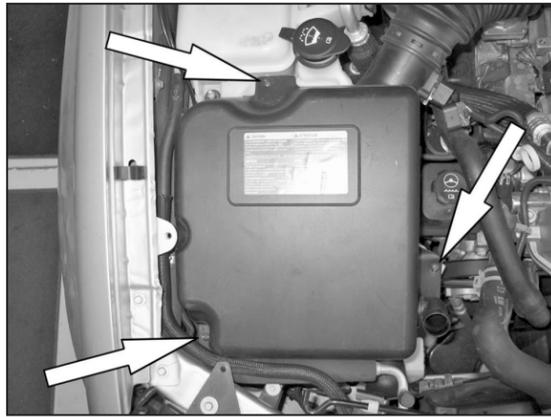
4. Loosen the three screws which secure the upper air box housing.
