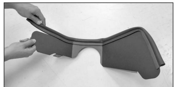
9. Install the provided edge trim onto the heat shield as shown.
