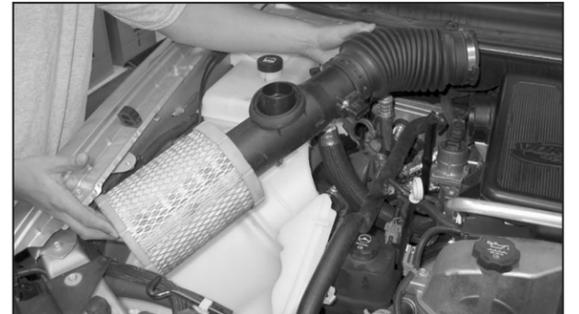
7. Loosen the hose clamp which secures the intake tube to the intake plenum and then remove the complete intake system as shown.
