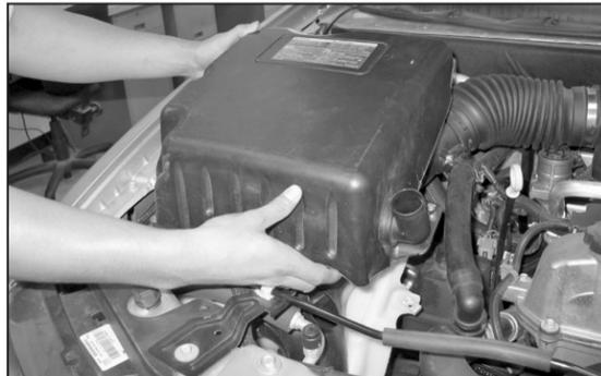
5. Remove the upper air box housing from the vehicle as shown.
