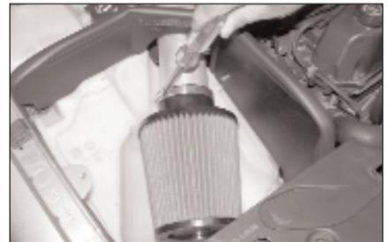
20. Install the K&N® air filter onto the K&N® intake tube and secure using the provided hose clamp as shown.
