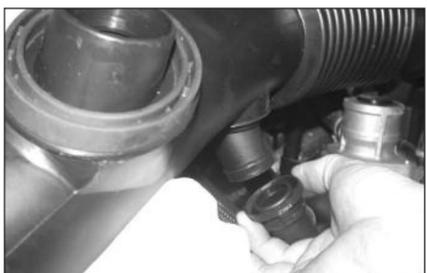
7a. On vehicles with air injection squeeze release ring then remove air injection line from intake tube.
