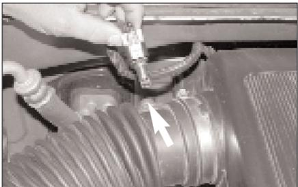
3. Remove the air temperature sensor from the stock intake tube as shown.
