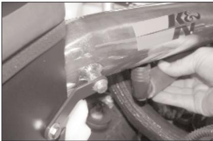
16b. On vehicles with air injection, install the 90 degree fitting into the vent line then mark the intake tube where the fitting lines up with tube, then remove intake tube from vehicle.
