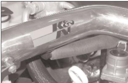
16d. Re-install the intake tube onto the vehicle, then install the 90 degree fitting into the grommet on the intake tube as shown.
