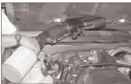
8. Remove the complete air intake assembly as shown.
