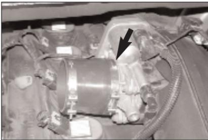
13. Install the silicone hose and hose clamps onto the throttle body as shown. The hose clamp on the throttle body may be tightened at this time.
