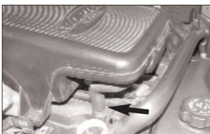
7. Loosen the hose clamp at the throttle body, then, lift the resonator upwards and disconnect the crank case vent hose as shown.
