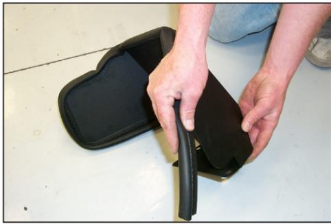
10. Install the edge trim onto the heat shield as shown.
