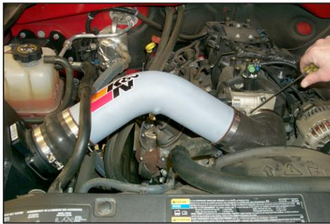
16. Install the K&N® intake tube into the angled hose, then, slide the other end into the hump hose. Adjust everything for best fit and clearance and tighten all hose clamps as shown.
