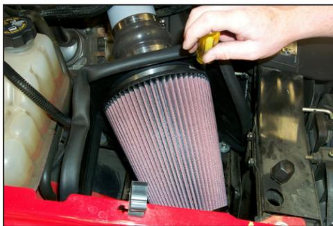
18. Install the K&N® air filter onto the mass air adapter and secure it with the provided hose clamp as shown.
