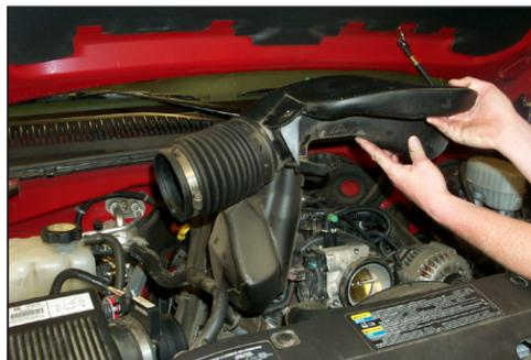
5. Loosen the hose clamps at the throttle body and at the mass air sensor, then remove the stock intake tube as shown.
