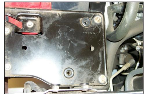
9. Install the rubber mounted studs as shown and tighten firmly by hand.
