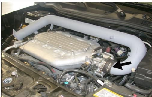
13. Install the K&N® Intake tube into the silicone hose on the throttle body as shown.
