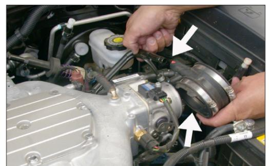
8. Remove the rubber coupler from the throttle body and disconnect the crank case vent as shown.
