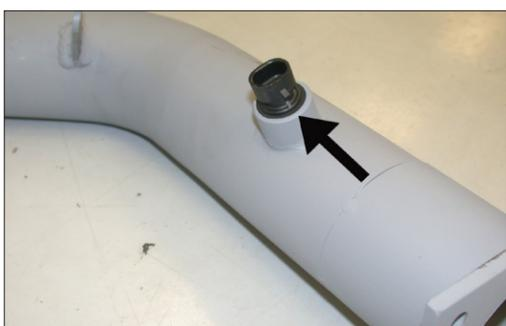
12. Install the air temperature sensor into the silicone hose as shown.
