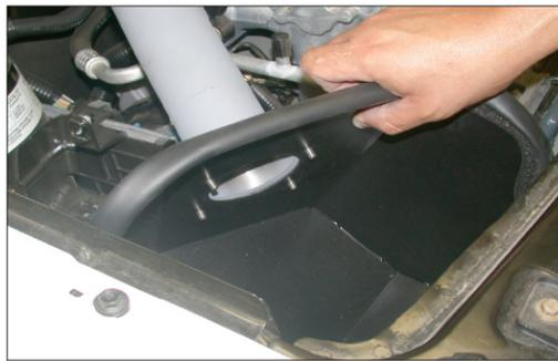
18. Install the heat shield onto the flange as shown.
