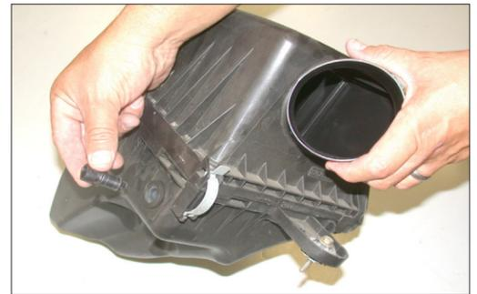
7. Remove the air temperature sensor from the air cleaner as shown.
