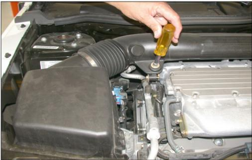
2. Remove the bolt that secures the air intake tube as shown.
