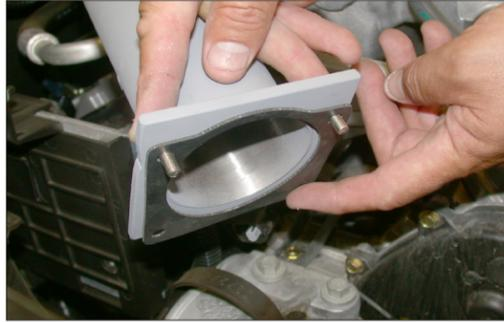
17. Install the hardware and one of the provided gaskets onto the intake tube flange as shown.
