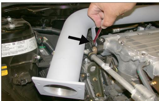
15. Secure the bracket to the stud using the nut removed in step 9 but do not tighten completely at this time.
