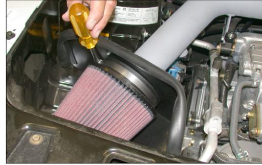
22. Install the Air Filter onto the filter adapter and secure it with the provided hose clamp as shown. **NOTE: The air filter will have to be compressed/ squeezed and slid into the inner fender.**
