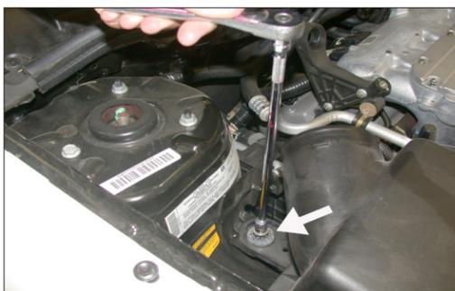
5. Loosen and remove the bolt at the back of the air cleaner as shown.
