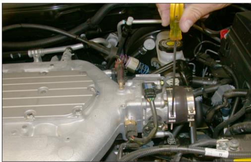
10. Install the silicone hose and hose clamps onto the throttle body as shown.
