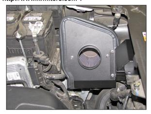
11. Install the heat shield/filter assembly into position so that the mounting studs engage the mounting grommets.
