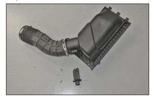
13. Remove the two screws securing the inlet air temperature sensor to the factory intake tube and then remove the sensor.
