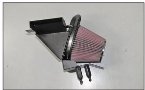
10. Install the air filter onto the filter adapter and secure with the provided hose clamp.
