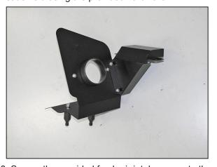
8. Secure the provided fresh air intake scoop to the heat shield using the provided hardware.
