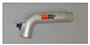
14. Install the inlet air temperature sensor into the K&N® intake tube and secure with the provided hardware.
