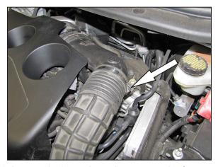
3. Loosen the hose clamp that secures the factory intake hose to the turbo inlet pipe.
