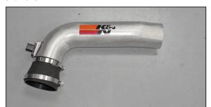
15. Install the step coupler hose (084055) onto the K&N<sup>®</sup> intake tube as shown. Do not tighten the hose clamp at this time.
