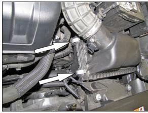
4. Release the two upper air filter housing retaining clips and then remove the upper air filter housing and intake hose assembly.
