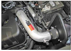
17. Install the K&N® intake tube assembly into the coupler at the turbo inlet tube, then slide the step coupler onto the filter adapter. Adjust the tube for best fit and secure the hose clamps.
