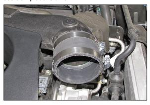
16. Install the coupling hose (08711) onto the turbo inlet pipe and secure with the provided hose clamp.
