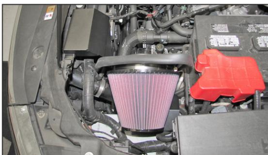
11. Install the K&N® filter/heat shield assembly so the stand-offs insert into the air box mounting grommets. Align the K&N® fresh air intake with the factory mounting holes and secure with the factory bolts removed in step #5.
