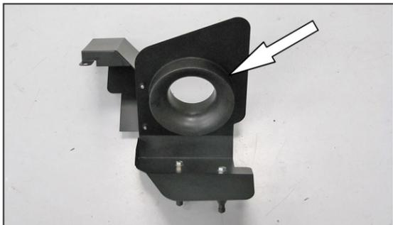
8. Install the filter adapter onto the heat shield as shown using the provided hardware.
