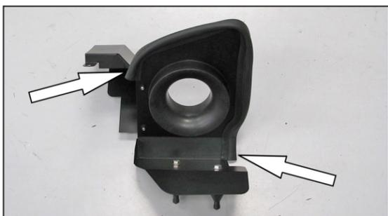
9. Install the provided edge trim onto the heat shield as shown.
