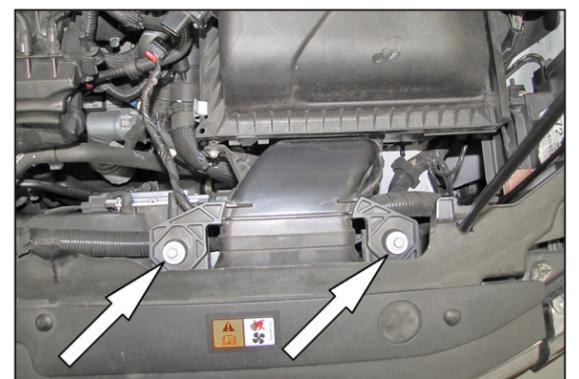
5. Remove the two bolts that secure the fresh air intake to the core support and then lift up and remove the complete intake assembly.
