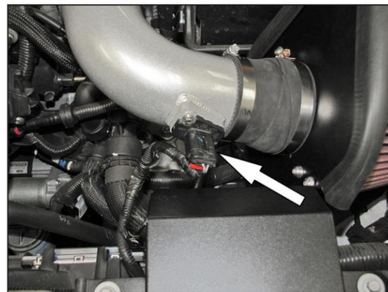
17. Reconnect the inlet air temperature electrical connection.
