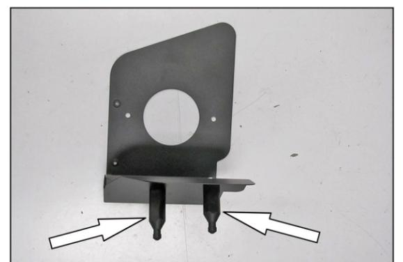
6. Install the two provided stand offs onto the heat shields using the provided hardware.
