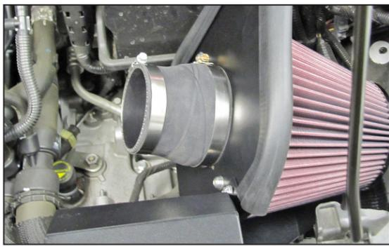
12. Install the provided step hose (084055) onto the filter adapter and secure with the provided hose clamp.
