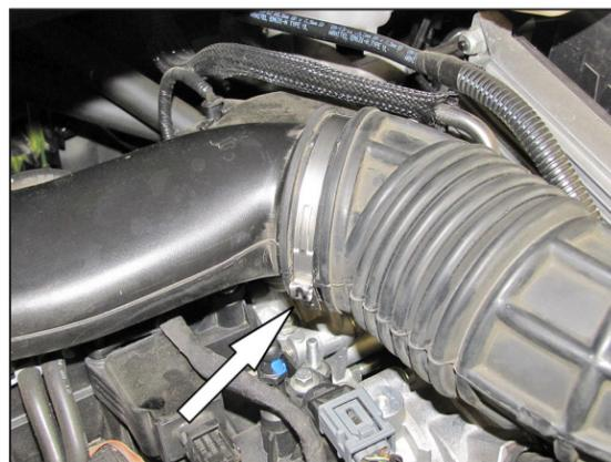
4. Release the hose clamp that secures the intake hose to the intake tube.
