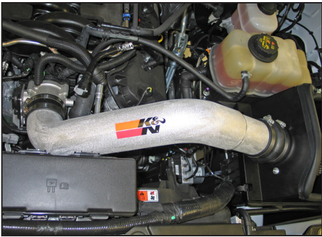
19. Install the K&N® intake tube assembly into the silicone hose attached to the filter adapter and then into the silicone hose on the throttle body. Secure with the provided hose clamps.
