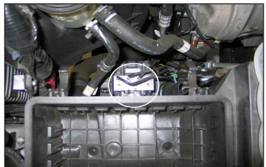
8. Remove the center upper airbox retaining clip from the lower airbox.
