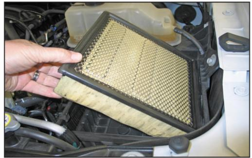
7. Remove the air filter from the lower airbox.
