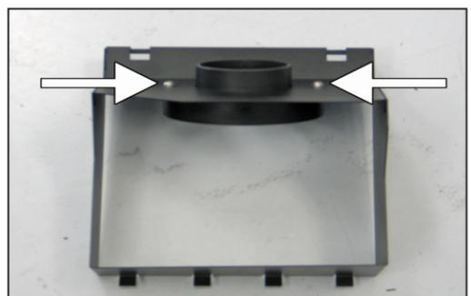
9. Install the K&N® filter adapter into the heat shield as shown. Secure with the provided hardware.
