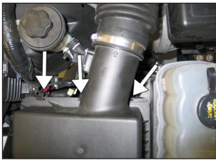
5. Release the three retaining clips that secure the upper airbox to the lower airbox.
