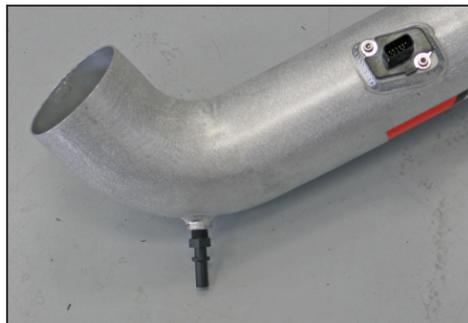
19. Install the provided crankcase vent fitting into the K&N® intake tube as shown.
