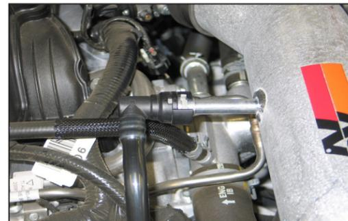
25. Connect the factory crankcase vent tube to the intake tube as shown.
