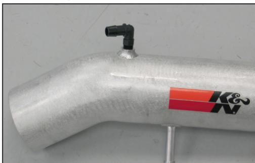
18. Install the 90° vent fitting into the intake tube as shown.
