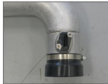
21. Install the mass air sensor into the intake tube and secure with the provided hardware.
