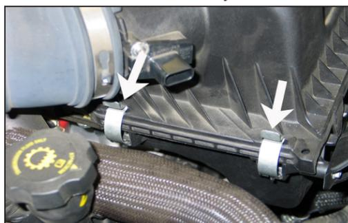
6. Release the two upper airbox latches shown.
