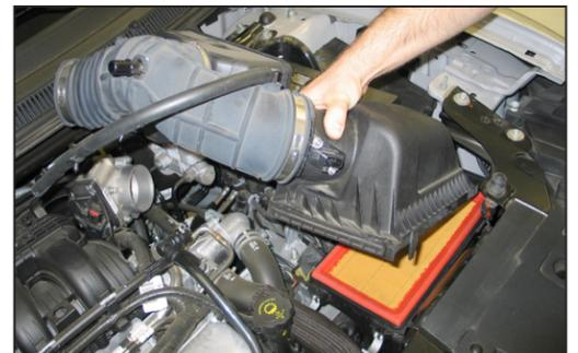
7. Disconnect the factory intake tube from the throttle body, then remove the upper airbox and intake tube from the vehicle.
