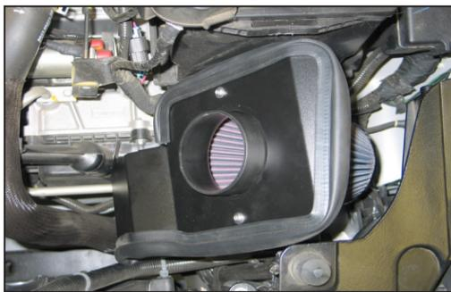
16. Set the heat shield onto the rubber mounted studs and then secure with the provided hardware. Install the K&N® air filter onto the adapter and secure with the provided hose clamp.
