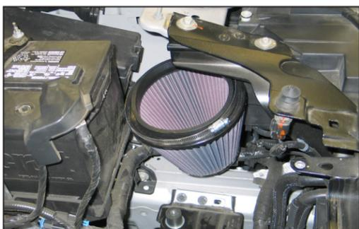
15. Set the K&N® air filter into the engine compartment as shown.
