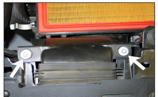
9. Remove the two bolts that secure the fresh air duct to the core support.
