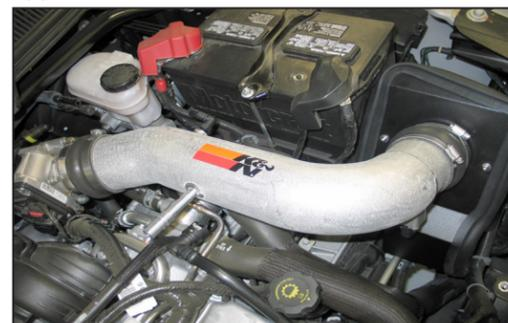
24. Install the intake tube into the silicone hose at the throttle body and onto the filter adapter, then secure with the provided hose clamps.
