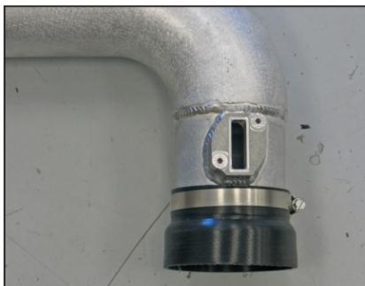
19. Install the remaining silicone hose (084073) onto the intake tube and secure with the provided hose clamp as shown.
