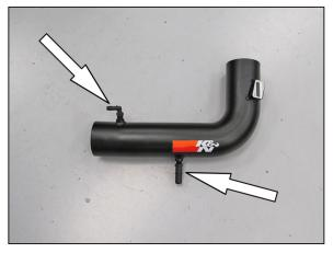
17. Install the provided 90° NPT vent fitting and NPT quick disconnect fitting into the K&N® intake tube as shown.
