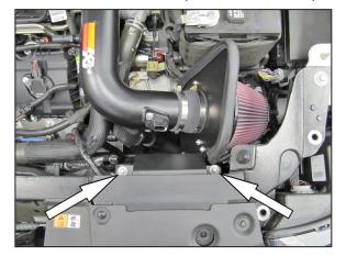
21. Secure the K&N® fresh air intake scoop to the core support with the factory bolts removed in step #7. Reinstall the factory plastic cover.
