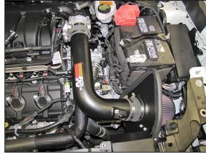
20. Install the K&N® intake tube assembly into the silicone hose at the throttle body and then at the filter adapter, align the tube and heat shield for best fit and then secure with the provided hose clamps.
