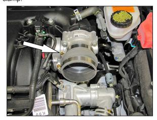
16. Install the provided silicone hose (08171) onto the throttle body and secure with the provided hose clamp.
