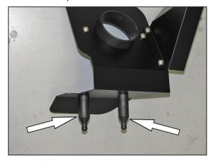
11. Install the two provided mounts onto the heat shield as shown using the provided hardware.
