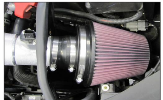
24. Install the filter assembly onto the intake tube and secure with the provided hose clamp.
