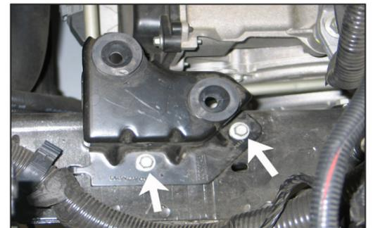
8. Remove the two bolts which secure the airbox mounting bracket to the inner fender.
