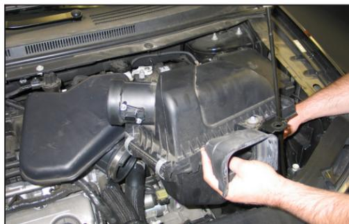
6. Remove the airbox from the vehicle.
