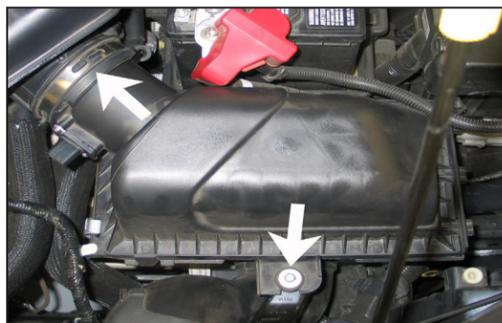
5. Loosen the hose clamp which secures the intake hose to the airbox. Remove the airbox mounting bolt shown.
