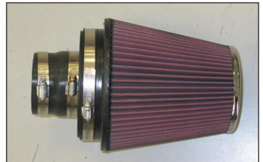
23. Install the silicone (084091) hose onto the filter adapter and secure with the provided hose clamp.
