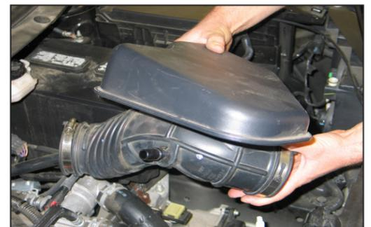
7. Loosen the hose clamp which secures the stock intake tube to the throttle body and then remove the intake tube from the vehicle.
