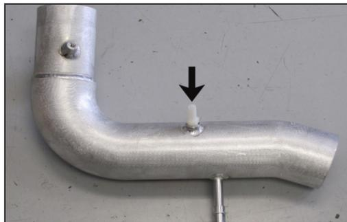
18. Install the provided 1/4npt fitting into the K&N® intake tube as shown.
