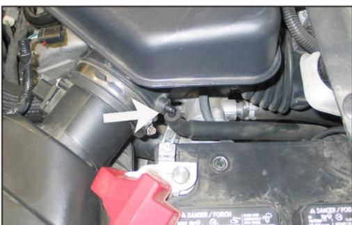
3. Disconnect the EVAP hose shown from the intake tube.
