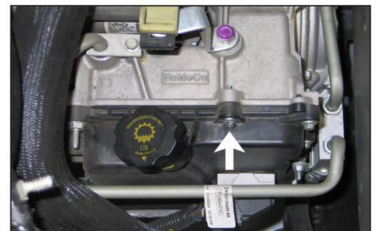
9. Remove the transmission pan bolt shown.
