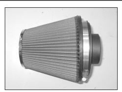
28. Install the air filter adapter into the K&N® air filter as shown and secure with the provided hose clamp.
