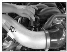
26. Install the supplied shorter crankcase vent hose onto the fitting on the valve cover and then onto the on the K&N® intake tube as shown.
