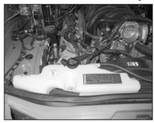
11. Reinstall the coolant recovery tank and secure with the factory bolts removed in step #8.
