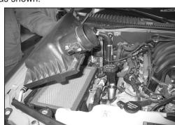
7. Unlatch the three airbox lid latches and then remove the lid from the vehicle.
