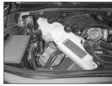
9. Lift and position the coolant recovery tank on the engine to gain access to the lower airbox.
