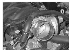
22. Install the silicone hose (08630) onto the throttle body and secure with the provided hose clamp.
