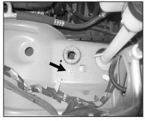
13. Remove the washer bottle mounting bolt shown
