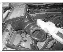
10. Lift up the lower airbox housing to dislodge it from the mounting grommets and then remove the lower airbox housing from the vehicle.
