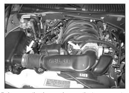
5. Loosen the hose clamps that secure stock intake tube to the throttle body and airbox shown.
