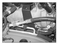
16. Install the tube mounting bracket onto the valve cover and secure with the factory valve cover mounting bolt and the supplied hardware as shown.
