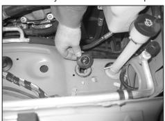
12. Remove the front lower airbox mounting grommet shown.
