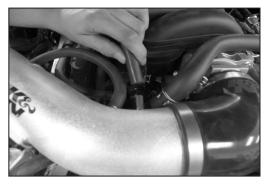
27. Install the supplied brake booster vent hose onto the factory fitting and then connect the other end to the fitting on the K&N® intake tube as shown.
