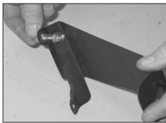
15. Insert the bolt removed in step #14 through the keyhole in the tube mounting bracket as shown.
