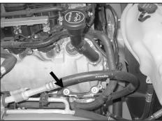
14. Remove the valve cover mounting bolt shown. **NOTE: this bolt will be reused.**
