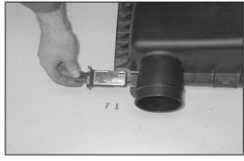
23. Remove the two screws that secure the mass air sensor to the stock airbox and then remove the mass air sensor.
