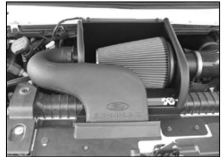
32. Install the factory fresh air scoop onto the heat shield and then latch it into the cut out and factory opening as shown.
