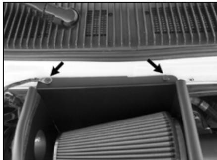
30. Using the factory bolts removed in step #3, secure the heat shield to the cowl.
