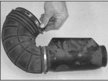
8a. On vehicles equipped with an external air temperature sensor; remove the air temperature sensor from the stock intake tube.
