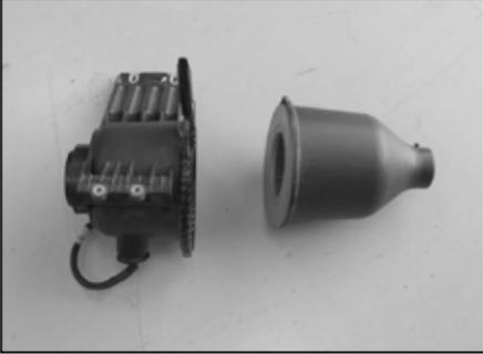
9. Unlatch the clam shell connector and separate the air filter assembly as shown.
