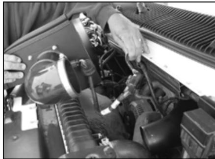
28. Set the filter assembly on top of the radiator assembly, reconnect the mass air sensor secondary connection and then set the filter assembly into position on the cowl and radiator core support.
