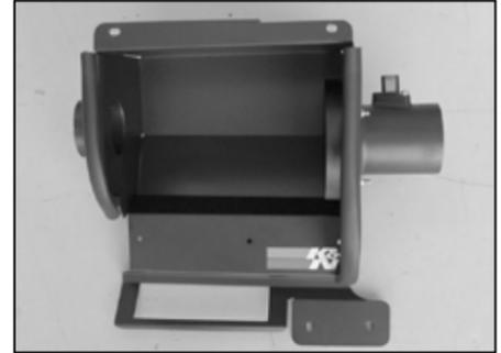
21. Install the mass air sensor assembly onto the studs and secure with the provided nuts and washers.
