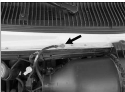
3. Remove the two bolts that secure the air filter assembly to the cowl.
