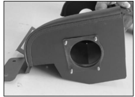
20. Install the remaining mass air sensor gasket onto the studs of the filter adapter protruding through the heat shield.
