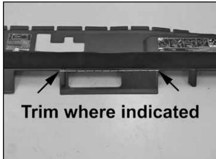
31a. On vehicles that the cowl cover conceals the air box mounting bolts, trim the cover as indicated by the dashed line so that the cover will sit flat onto the cowl.
