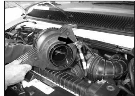
6. Lift up the air filter housing and unhook the mass air sensor secondary connector from the housing. Then disconnect the mass air sensor secondary connection and remove the filter assembly from the vehicle.
