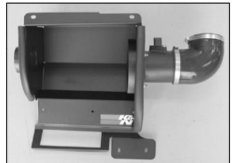
23. Install the silicone hose (084088) onto the mass air sensor housing and secure with the provided hose clamp.
