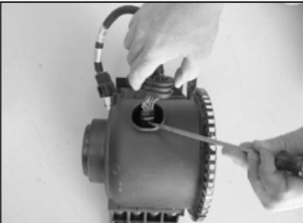
10. Pull back the rubber plug to gain access to the primary mass air sensor connection. Using a small screw driver, release the locking tab and disconnect the mass air sensor electrical connection.
