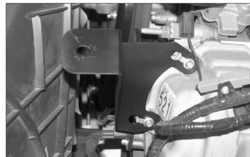
25. Install the tube mounting bracket onto the valve cover using the factory bolts. Do not completely tighten the bolts at this time.
