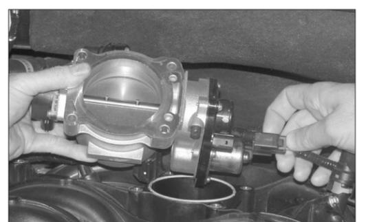
9. Lift throttle body from intake manifold. Then disconnect throttle body motor electrical connection.
