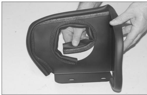
16. Install the short edge trim into the hole in the heat shield as shown.
