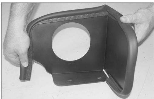
15. Install the long edge trim onto the heat shield as shown.
