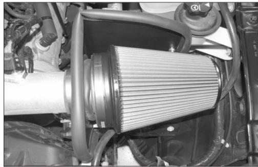
36. Install the K&N® air filter assembly onto the K&N® intake tube as shown and secure with the provided hose clamp.
