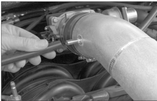
29. Install the provided silicone vent hose onto the valve cover and onto the K&N® intake tube as shown.
