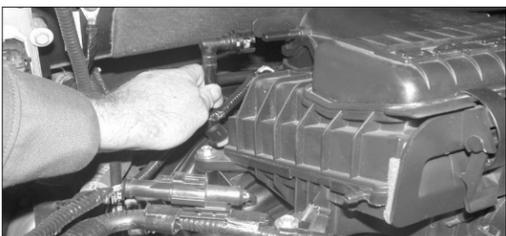
4. Rotate crank case vent hose locking ring and pull crank case vent hose off of air filter housing. Unhook wiring harness retaining clip from air box.
