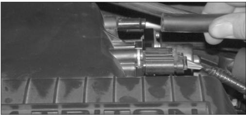
2. Disconnect the brake booster vent line from the air filter housing as shown.
