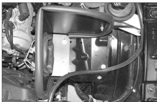
20. Install the heatshield as shown and secure with the provided hardware.
