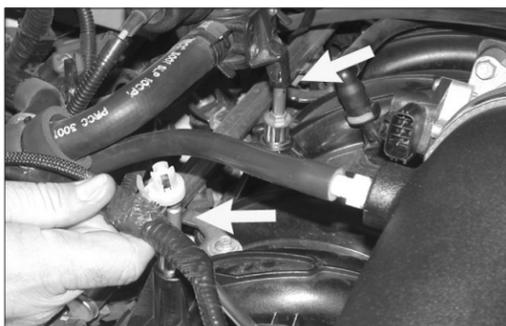
32. Re-install the heater control valve and wiring harness mounting clips onto the air box mounting studs as shown.
