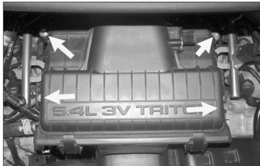
6. Remove the four air box mounting bolts shown with a 10mm socket.
