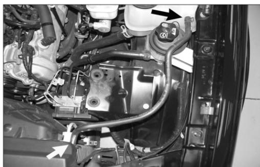
13. Loosen the coolant recovery hose, hose clamps, and then remove the factory recovery hose shown. Be sure to catch any coolant, which flows out of the radiator during hose removal.
