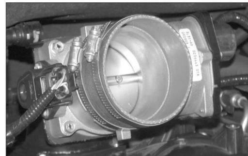
26. Install silicone hose (#08630) onto the throttle body with the provided hose clamps as shown.
