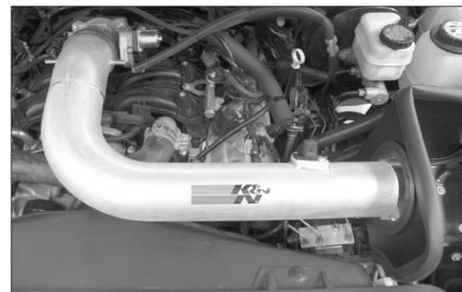
27. Install the K&N® intake tube onto the throttle body and position so that it lines up with the tube mounting bracket installed in step #25. Secure the intake tube with the provided bolt and hose clamp.
