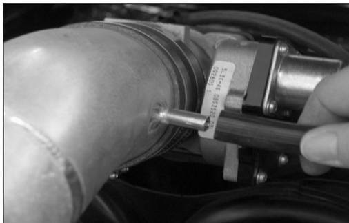
30. Connect the factory brake booster vent hose to the K&N® intake tube and secure with the provided hose clamp.
