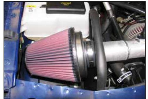
24. Install the air filter and secure with hose clamp provided.
