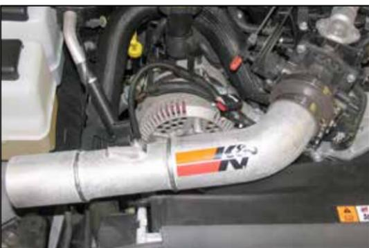
15. Install the K&N® intake tube into the throttle body and secure the bracket in place on the alternator with the bolt removed in step #14.
