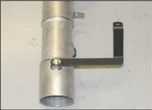
13. Install the provided tube mounting bracket (010081) onto the K&N® intake tube with the provided hardware as shown.
