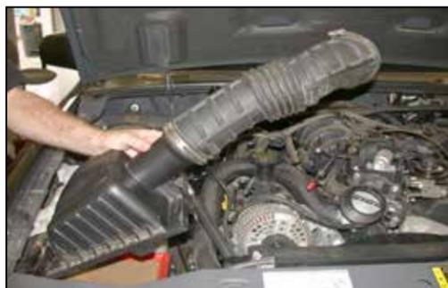
6. Loosen the hose clamp which secures the intake tube to the throttle body, release the two clam shell clamps which secure the upper air box lid and then remove the air box lid and intake tube from the vehicle.
