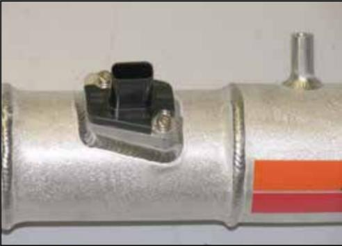
12. Using the provided mounting screws, install the mass air sensor into the intake tube as shown.
