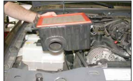
7. Pull firmly up on the lower air box housing to dislodge from the mounting grommets and remove lower air box from the vehicle.
