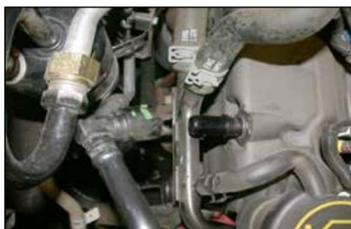
5. Depress the green locking tab and disconnect the crank case vent line from the valve cover as shown.
