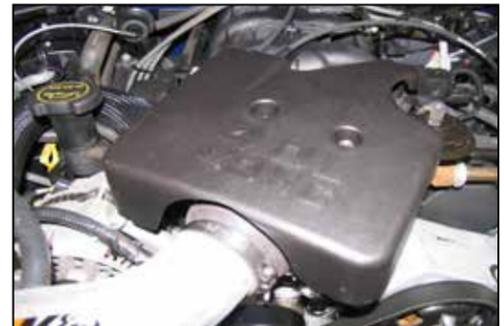
25. Reinstall the engine cover and secure with the factory mounting bolts.
