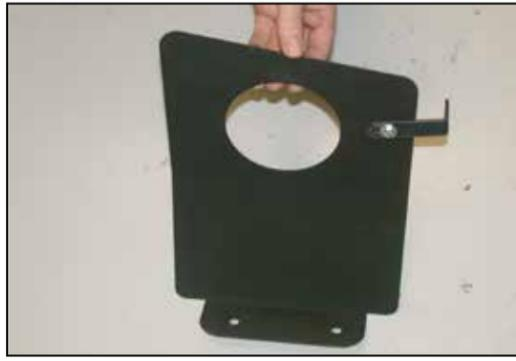
16. Install the heat shield mounting bracket (070742) onto the heat shield with the provided hardware as shown.
