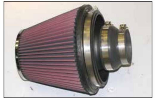
23. Install the provided silicone hose (084093) onto the air filter assembly and secure with the provided hose clamp as shown.
