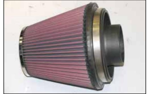
22. Install the provided adapter into the K&N® air filter and secure with provided hose clamp as shown.
