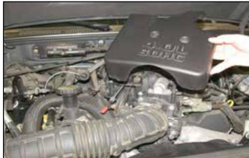
4. Remove the engine cover from the engine.
