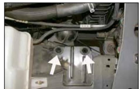
9. Remove the two air box mounting grommets from the mounting plate shown.
