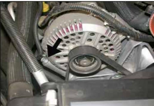
14. Remove the front lower alternator mounting bolt shown.
