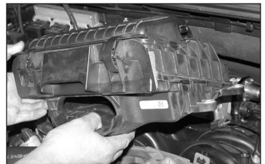
8. Pull firmly upwards to remove the air cleaner as shown.
