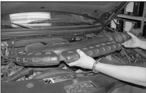
3. Pull firmly on the stock intake tube to release it from the stock air cleaner and the inner fender, then, remove the stock intake tube as shown.
