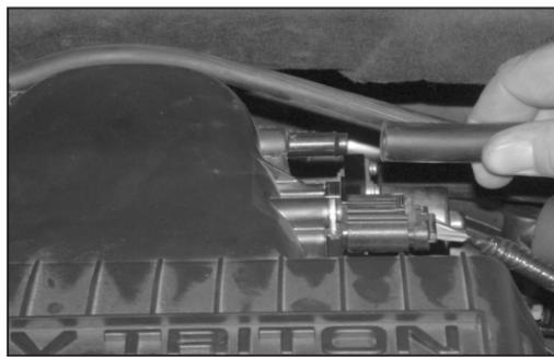
5a. Disconnect the brake booster vent line from the air filter housing as shown.
