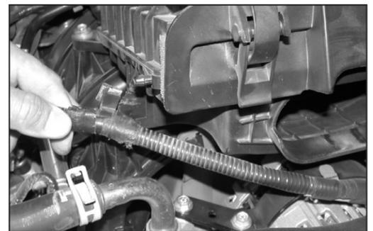
6. Unclip the wire harness from the air cleaner as shown.
