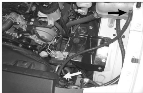
15b. Install the supplied coolant recovery hose and secure with the provided hose clamps.
