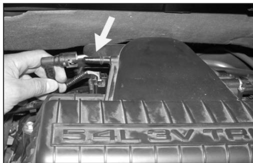
5. Disconnect the crankcase vent hard line from the air cleaner as shown.
