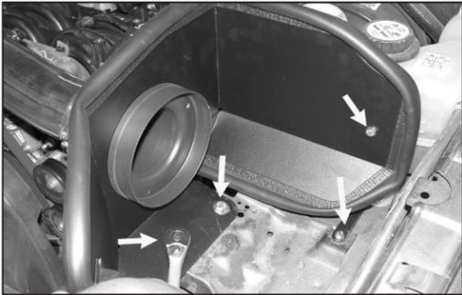
21. Adjust the heat shield for best fit and clearance, then, tighten all hardware at this time.
