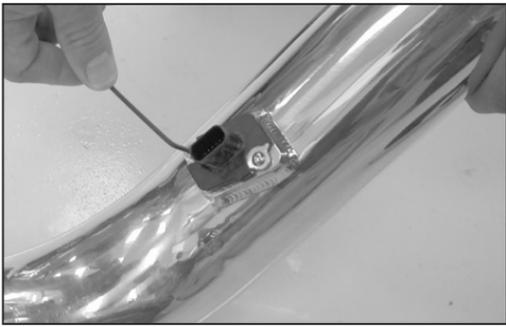
18. Install the mass air sensor into the K&N® Intake tube and secure with the provided hardware as shown.
