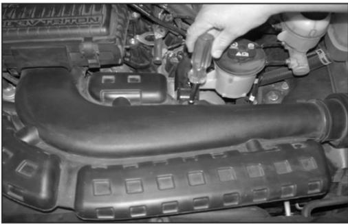
2. Remove the bolt that secures the intake tube to the power steering bracket as shown.
