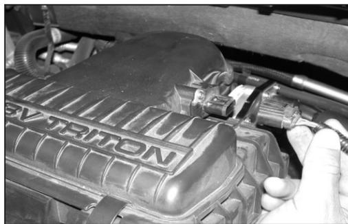
4. Disconnect the mass air sensor electrical connection as shown.
