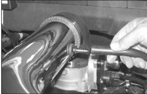
23a. On vehicles equipped with brake booster vent line install the provided hose mender into the grommet in the intake tube and connect the brake booster vent line to the hose mender.
