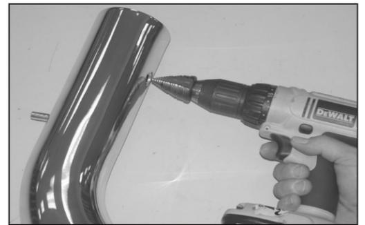
17b. Remove the intake tube and drill a 5/8" hole at the location marked in step #17a.
