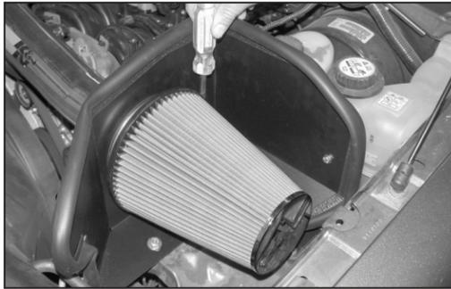
24. Install the K&N® air filter and tighten the provided hose clamp as shown.
