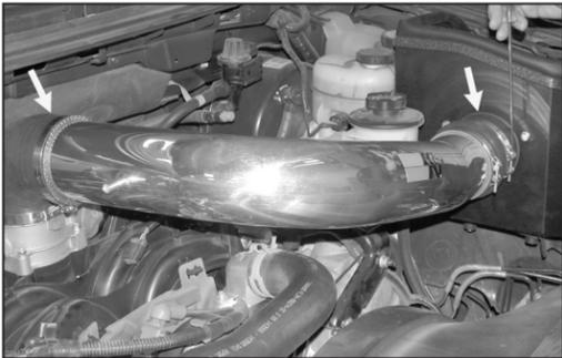
20. Slide the silicone hump hose onto the filter adapter, then, slide the other end into the 90° silicone hose, adjust everything for best fit and clearance and tighten all hose clamps as shown.
