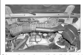
7. Loosen the hose clamps at the throttle body and at the mass air sensor, then, remove the stock intake tube as shown.
