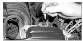
5. On vehicles with and intake resonator remove the bolt that secures the resonator to the engine bracket as shown.
