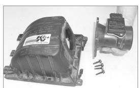
12. Remove the mass air sensor from the air cleaner cover as shown.
