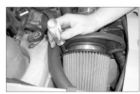
23. Slide the filter onto the mass air adapter and secure with the provided hose clamp as shown.
