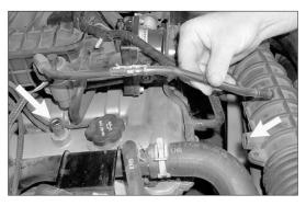
6. Remove the crank case vent hose from the vent on the cam cover and remove the other end from the vent on the stock intake tube as shown.
