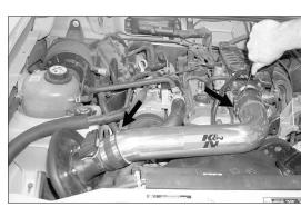
19. Slide the intake tube into the silicone hose at the throttle body and at the mass air sensor, adjust for best fit and tighten as shown.
