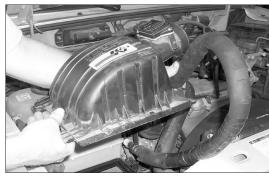
9. Unclip the air cleaner cover and remove as shown.
