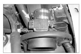
18. Install the silicone hose and hose clamps onto the mass air sensor and tighten as shown.
