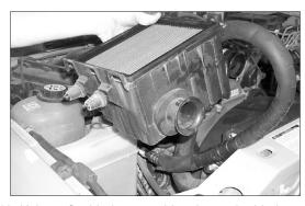
10. Using a flat blade screwdriver insert the blade between the air cleaner tray and the bottom of the lower air cleaner. Pry downward on the tray with the screwdriver while lifting upward on the air cleaner to release it from the stock grommets as shown.
