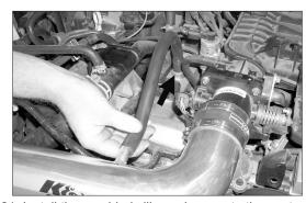
21. Install the provided silicone hose onto the vent on the cam cover, then, connect the other end to the vent on the intake tube as shown.
