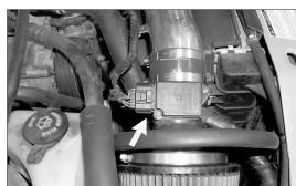
$25. \ \mbox{Reconnect}$  the mass air sensor electrical connection as shown.
