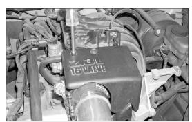
27. Install the throttle body cover and secure with the stock bolts as shown.
