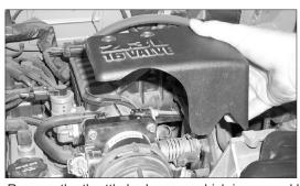
4. Remove the throttle body cover which is secured by two bolts as shown.
